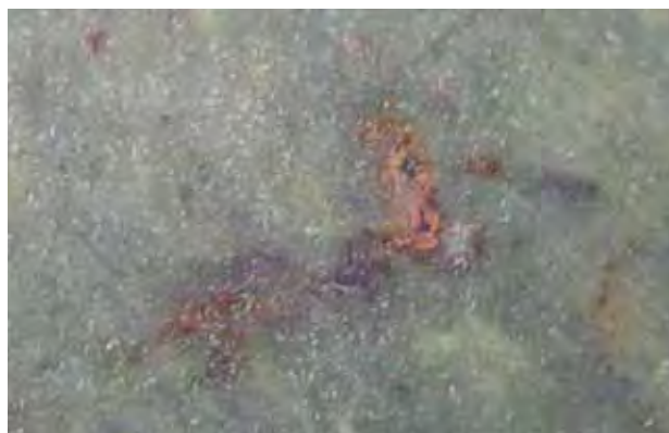
Figure 13. The metallic inclusions in this jadeite from Clear Creek, California, consist of native copper. The largest copper inclusion measures approximately 2 mm in longest dimension. Courtesy of S. Perry; photomicrograph by R. Merk, magnified 10×.
