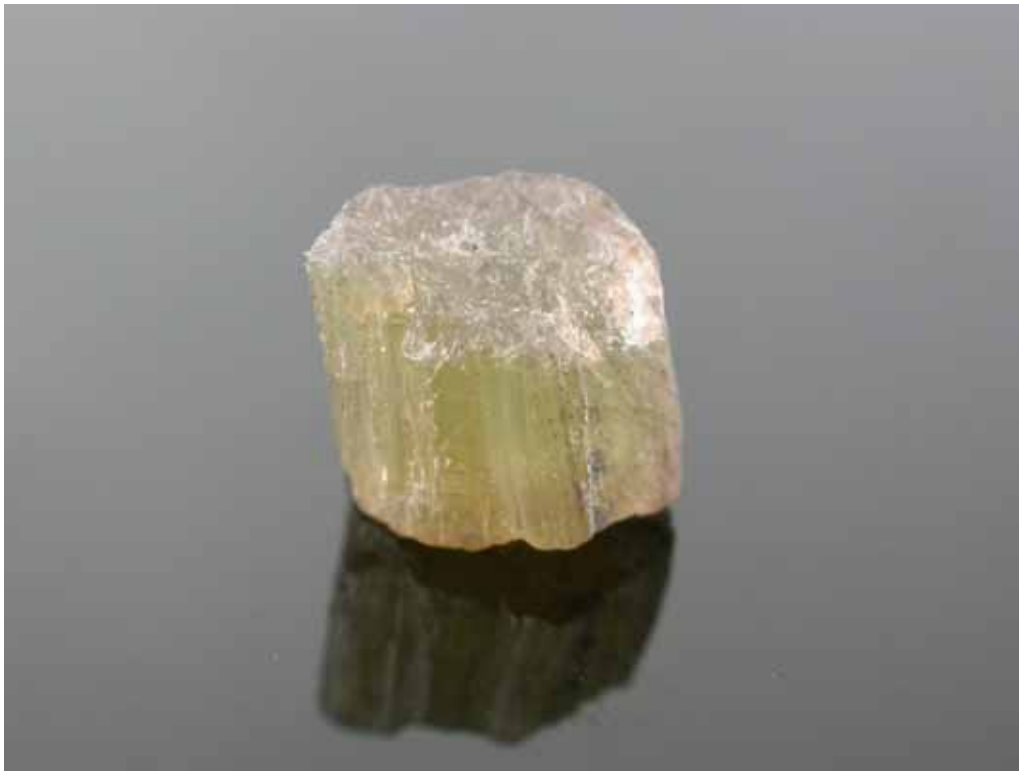
The andalusite specimens often showed prism faces intersecting each other at 90^\circ and exhibited striations parallel to the c-axis. Photo by G. Choudhary.
