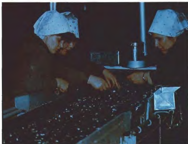
Figure 10. Highly trained workers sort out emeralds on a slow-moving conveyor belt at the Malysheva processing plant.
