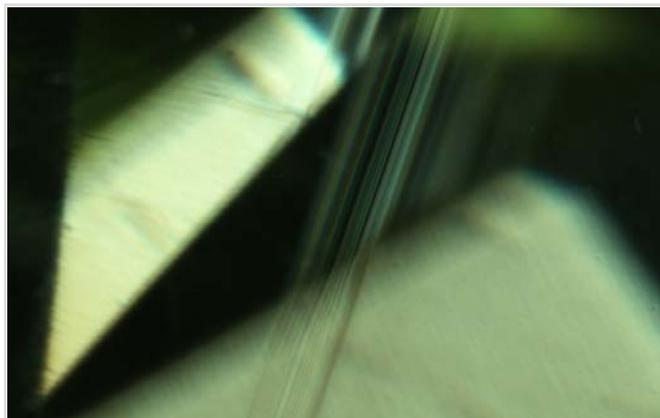
These trails of tiny particles are aligned along parallel growth zoning. The field of view is 1.45 mm across.
