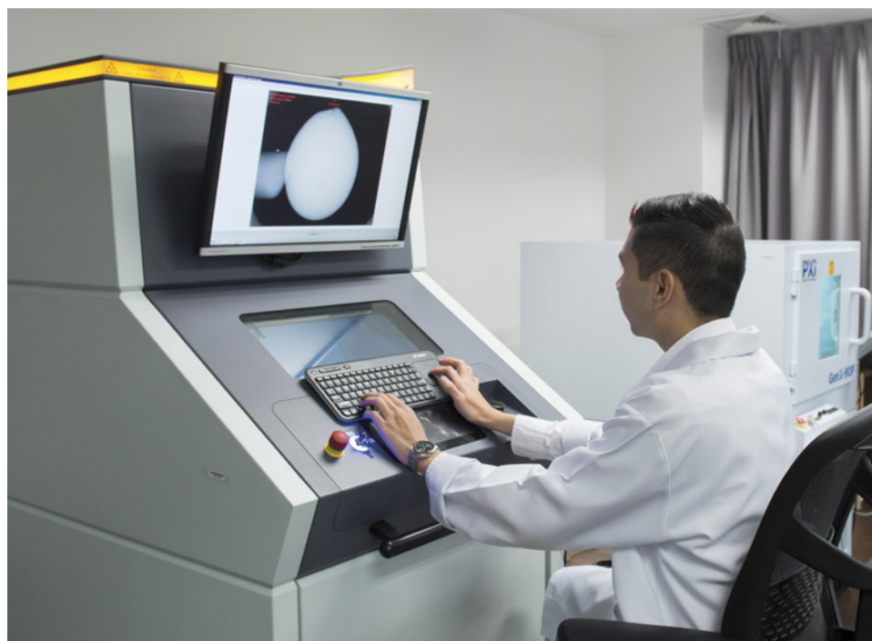
Figure 3. Modern gemological laboratories use real-time X-ray imaging systems to assess the transparency of gem materials, which is especially important for distinguishing natural from cultured pearls. Photo by Nuttapol Kitdee.
