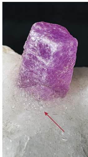
Figure 6. Left: Marble-hosted ruby specimens (ruby crystals ranging from 0.6 to 1.0 cm in height) reportedly mined from Hunza and acquired from the nearby local market. The natural specimen components have been artificially assembled with a resin-like adhesive. Right: In some specimens, the adhesive is well camouflaged and difficult to detect (indicated by arrow), especially if oiled. Photos by Talha H. Bakht.
