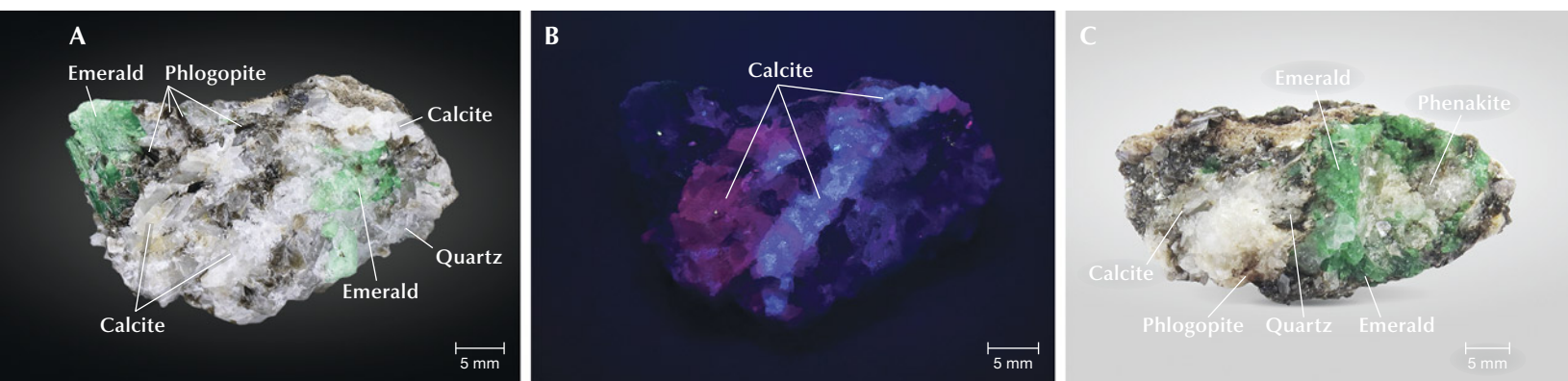
Figure 5. Two emerald specimens from quartz-calcite veins. A and B: Specimen containing emeralds and associated minerals such as white calcite, off-white quartz, and brown phlogopite. The calcite fluoresces moderately red (early crystallization, larger particles) and strongly blue (later filling crystallization, xenomorphic granular and smaller) under short-wave ultraviolet light. C: Emeralds with associated minerals such as white calcite, white or gray quartz, gray phenakite, and brown phlogopite. Photos by Sheng-Hao Zhu (A) and Yi Guo (B and C).
