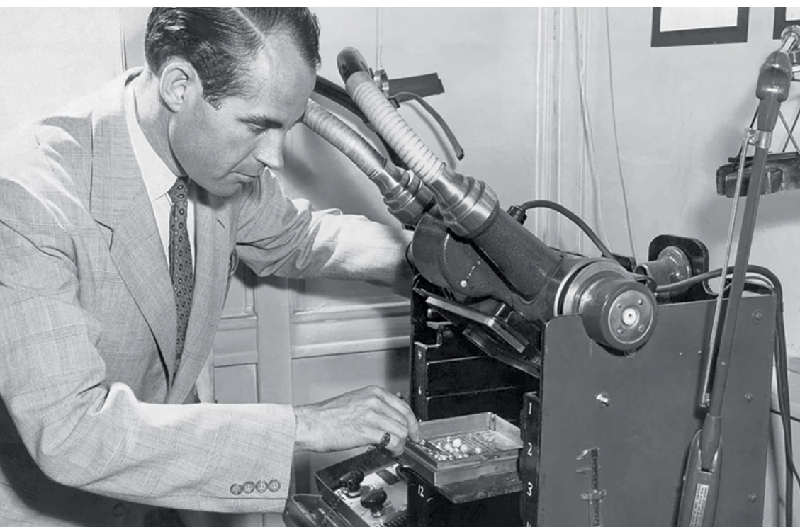
Figure 11. Robert Crowningshield preparing to X-ray several pearls at GIA's New York laboratory in the early 1950s.
