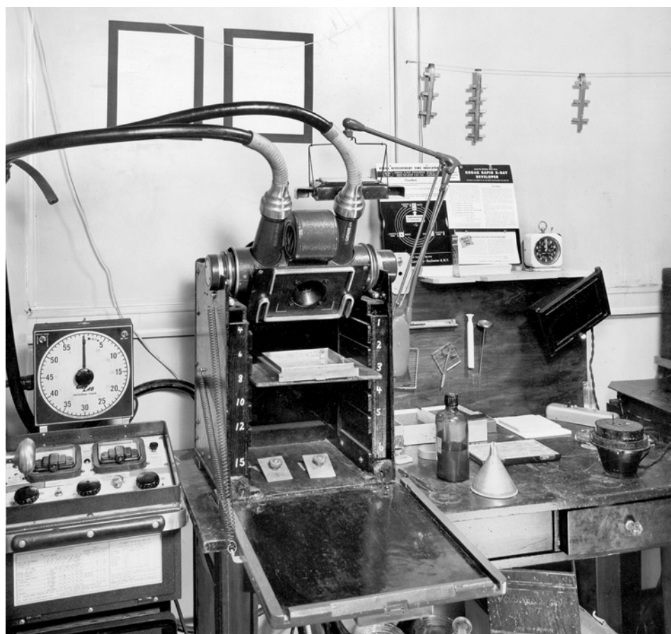
Figure 1. This specially adapted X-ray medical unit used by GIA during the 1950s features an automatic timer, a pearl tray, a lead glass protective cover, and accessories used in X-ray radiography.
