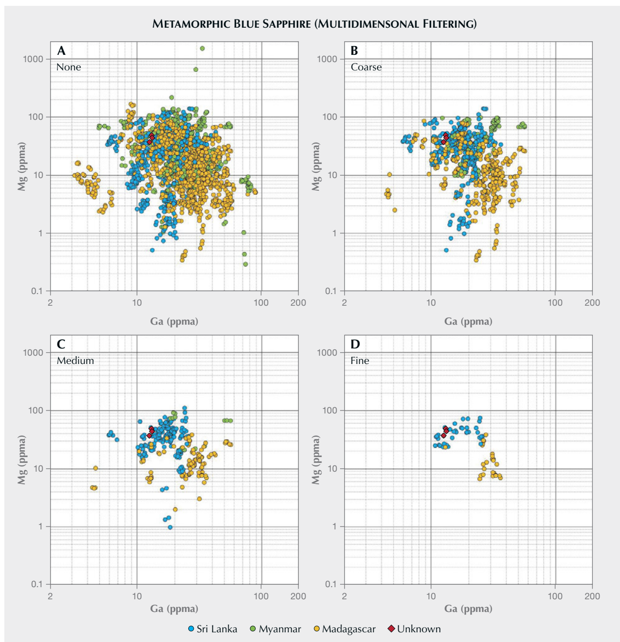
Figure 16. Visualization of the simultaneous multidimensional filtering process for metamorphic blue sapphire plots. A: The initial magnesium-gallium 2D plot prior to filtering. B: The magnesium-gallium 2D plot after coarse filtering using vanadium, iron, and titanium. C: The magnesium-gallium 2D plot after medium filtering. D: The magnesium-gallium 2D plot after fine filtering.
