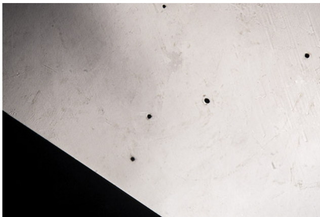
Figure 4. Examples of treatments documented in diamond. Left: Fracture filling in a feather on the table of a laboratory-grown diamond. Right: Reflective lighting displaying numerous laser drill holes in the table of a diamond. Photomicrographs by Nicole Ahline; fields of view 3.57 mm (left) and 4.79 mm (right).
