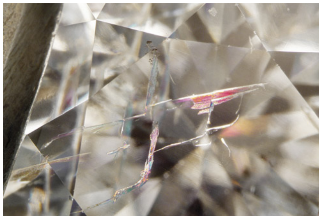
Figure 4. Examples of treatments documented in diamond. Left: Fracture filling in a feather on the table of a laboratory-grown diamond. Right: Reflective lighting displaying numerous laser drill holes in the table of a diamond. Photomicrographs by Nicole Ahline; fields of view 3.57 mm (left) and 4.79 mm (right).
