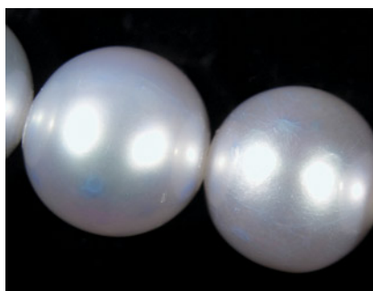
Figure 16. Left: Multiple blue color concentrations under the surface of one pearl; field of view 19.27 mm. Right: Blue dye concentration inside a fracture; field of view 2.34 mm.
