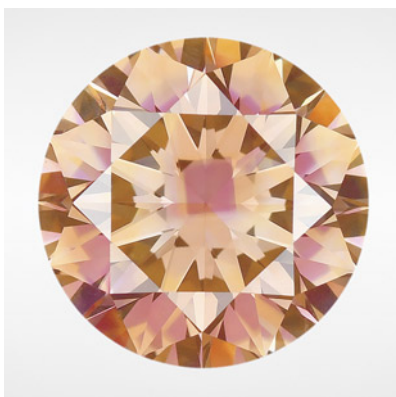
Figure 8. This 2.20 ct Fancy Deep brownish orange treated HPHT-grown diamond owes its distinctive appearance to multiple defect concentrations created within the various growth sectors.
