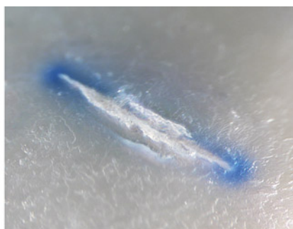
Figure 16. Left: Multiple blue color concentrations under the surface of one pearl; field of view 19.27 mm. Right: Blue dye concentration inside a fracture; field of view 2.34 mm.
