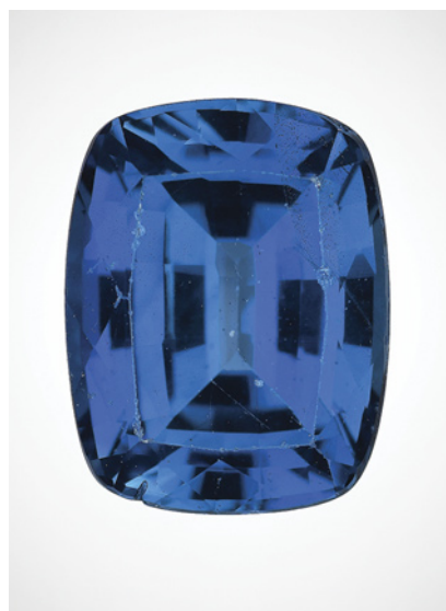
Figure 19. Face-up view of the 2.81 ct flame-fusion synthetic sapphire with flux fingerprints.
