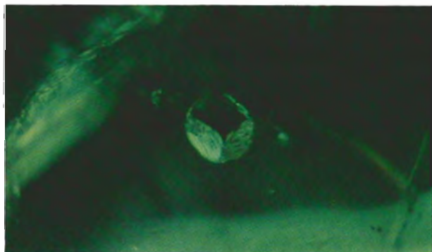
Figure 9. A well-formed pyrite inclusion in emerald from Santa Terezinha de Goiás. Magnified 45\times .
