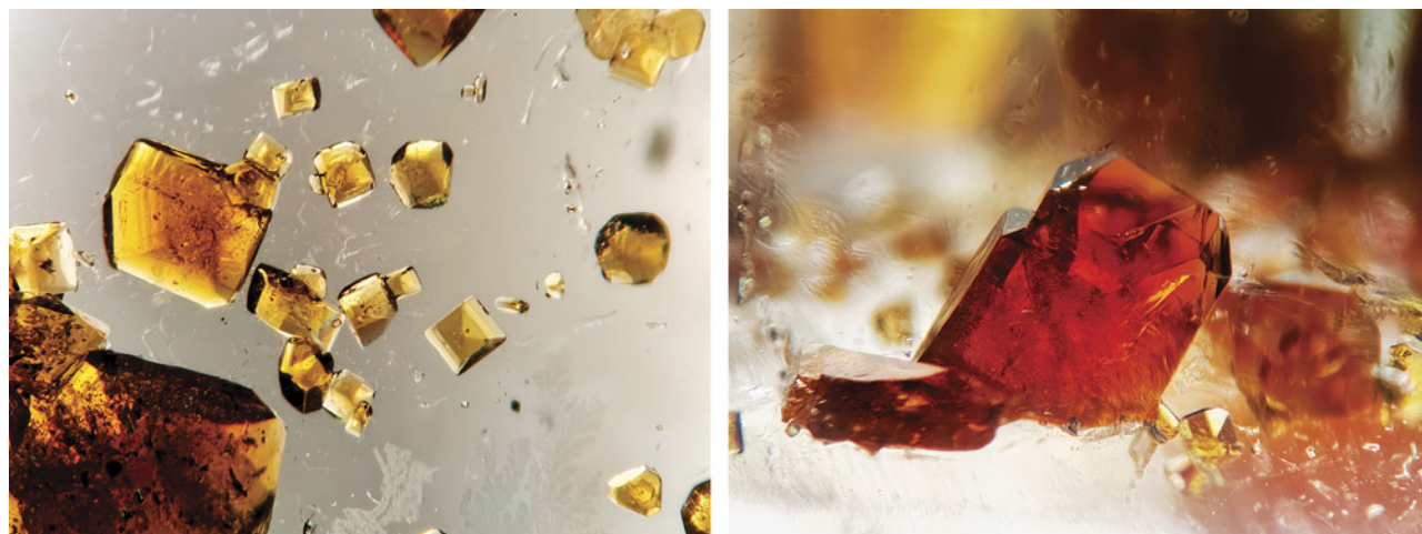
Figure 7. Left: Numerous orange-yellow to orange solid inclusions are visible within the transparent colorless quartz. Right: Closer observation reveals bright orange wedge-shaped crystals. Photomicrographs by Wingtak Lui; fields of view 5.1 mm (left) and 3.2 mm (right).
