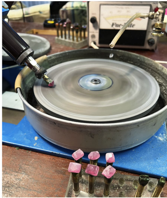
Figure 3. Converting a parcel of rhodochrosite rough into finished gems, from inspecting and grinding the rough (left) to the preformed and dopped rough (right). Courtesy of Ben Kho.
