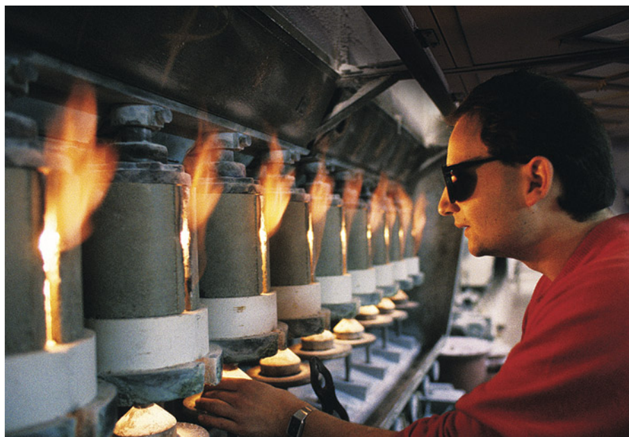
Figure 3. Drawing of a Verneuil (flame-fusion) apparatus (left) and a photo of flame-fusion crystal growth in the furnace (right). Photo courtesy of Hrand Djevahirdjian.
