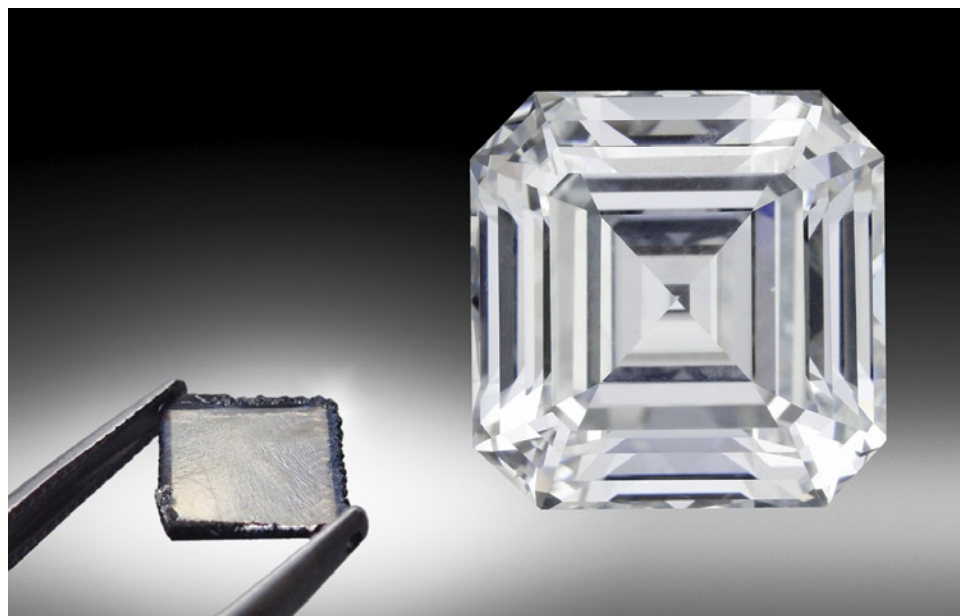
Figure 1. This 10.02 ct E-color, VS 1 -clarity emerald-cut diamond is an example of the great strides made in HPHT growth technology in the past two decades, as laboratory-grown diamonds have become an important sector of the gem diamond market. Photo by Johnny Leung. The as-grown CVD diamond plate (1.24 ct, 8.41 × 8.60 × 1.26 mm) was manufactured by GIA at its New Jersey research facility. Photo by Adrian Chan.
