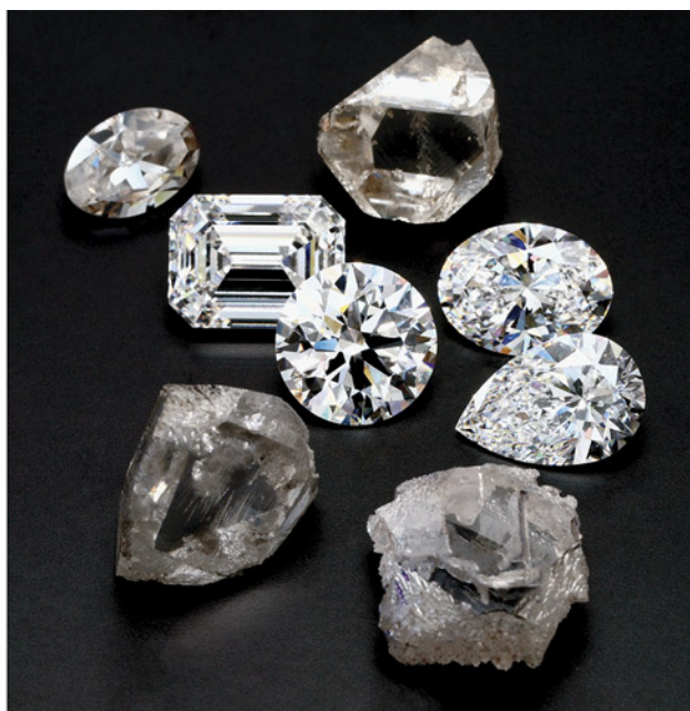
Figure 16. Planning CVD-grown rough diamond for cutting is done by computer-aided tools, which usually propose options for the cutters—in this case, the two round brilliants to be produced from one rough (left). Then cutters follow processes similar to those used for cutting and polishing natural diamonds (right, 3.16–5.44 ct). Courtesy of Clarity Diamond and HRA Group.
