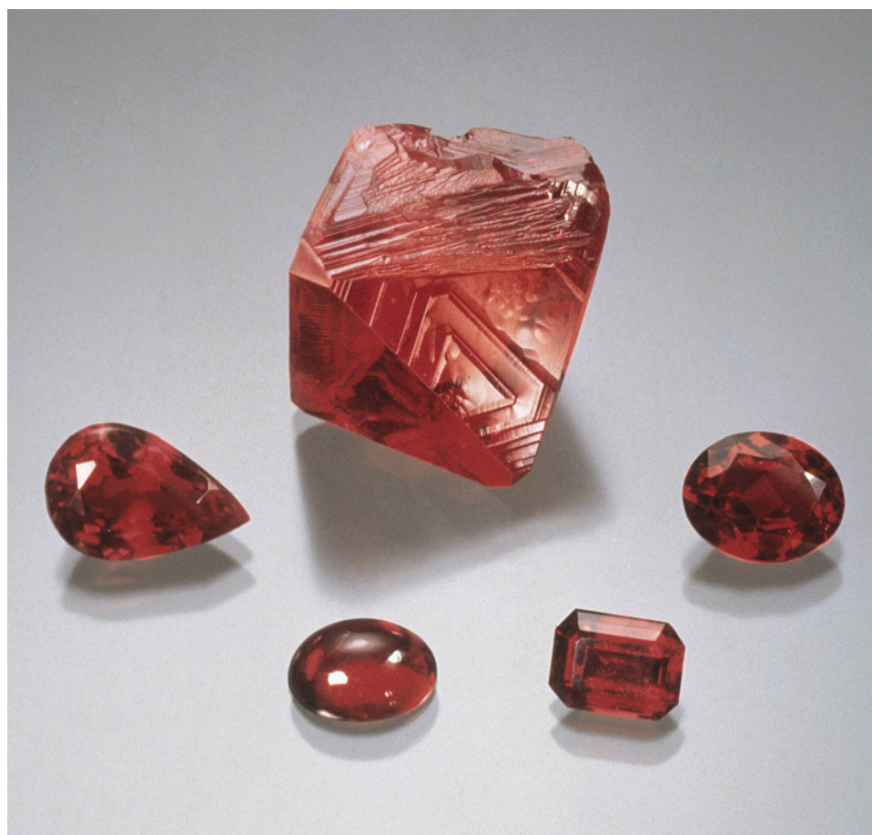
Figure 6. Flux-grown synthetic ruby produced by the Douros method. The rough rhombohedral crystal weighs 44.74 ct, and the cut stones range from 2.14 to 4.93 ct. Photo by Robert Weldon; courtesy of John Douros.
