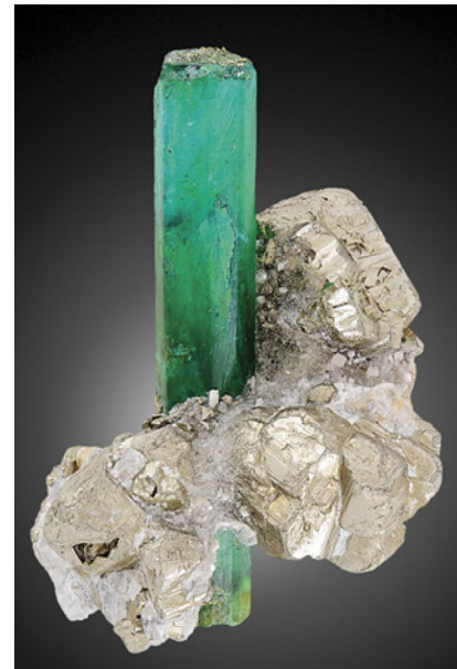
Figure 23. An assemblage of plastic and various minerals imitating rough emerald in matrix, measuring approximately 51.79 mm in height.
