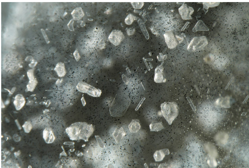
Figure 2. Negative crystals, film-like inclusions, and ilmenite were observed under magnification in the star aquamarine. Field of view 3.57 mm.
