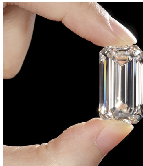
Figure 8. This 34.59 ct CVD-grown diamond ( 24.94 \times 13.95 \times 9.39 mm), produced by Ethereal Green Diamond in India, is the largest GIA has tested.
