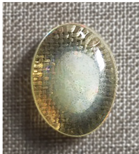
Figure 24. Left: The opal before treatment is semi-translucent white and shows a weak play-of-color. Right: After 36 hours of treatment, the opal becomes transparent light yellow, containing a white phantom. Photos by Le Ngoc Nang.
