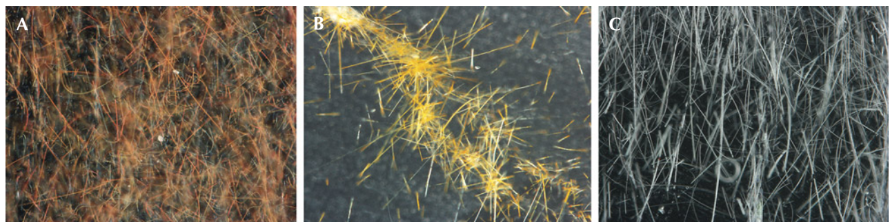
Figure 16. A: Fibrous inclusions in red rabbit hair quartz (sample R1). B: Needle-like inclusions in yellow rabbit hair quartz (sample Y2). C: The tubular inclusions in white rabbit hair quartz (sample W1). Photomicrographs by Shuqian Rui; fields of view 0.71 mm (A), 0.91 mm (B), and 1.26 mm (C).
