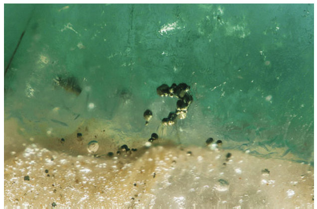
Figure 2. Cluster of pyrite crystals in emerald and matrix. Photomicrograph by Jessa Rizzo; field of view 1.99 mm.
