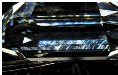
Figure 9. Observed with cross-polarized light was a strong tatami strain pattern with a dark gray color.
