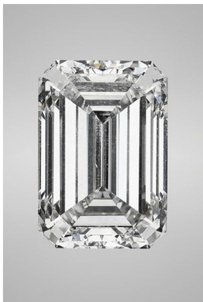
Figure 14. This 10.04 ct G-color CVD-grown diamond proved to have been HPHT treated.
