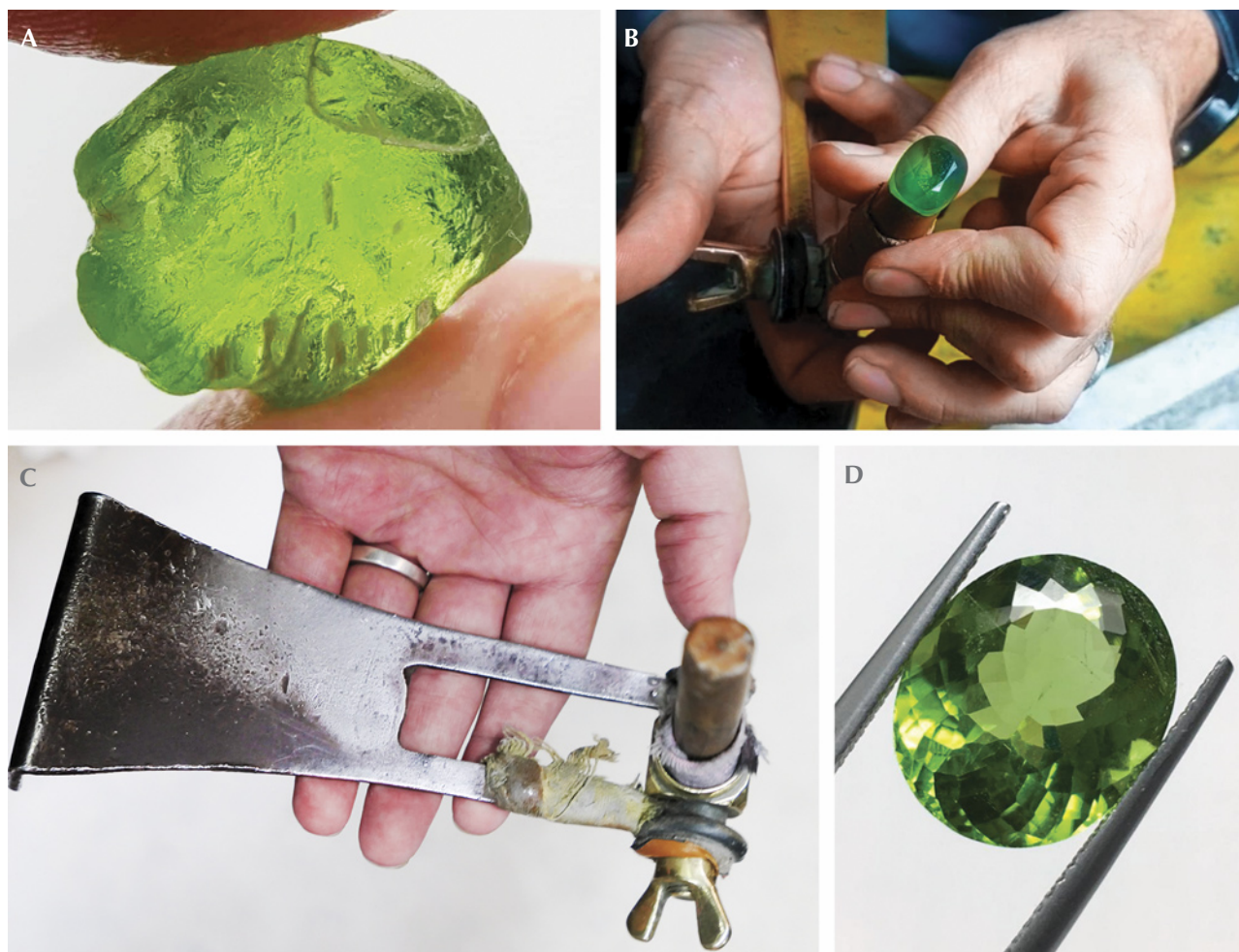
Figure 9. The angoora faceting process used by cutters at Namak Mandi. A: A rough peridot. B: The pre-formed, doped peridot. C: Instead of a modern faceting machine, local lapidaries use the angoora to save weight and maximize profits. D: The completed faceted peridot. Photos by Shakeel Anwar Khan.
