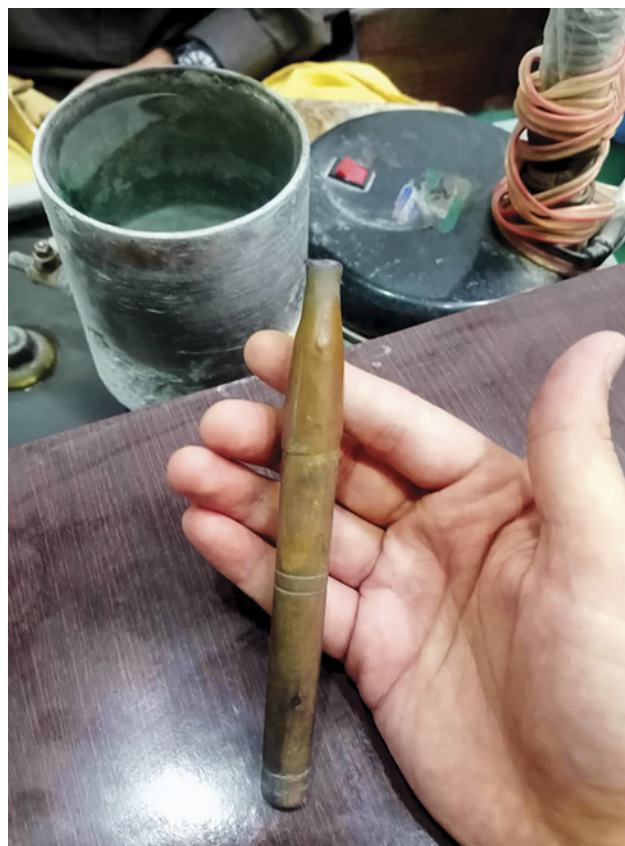
Figure 10. The khandee (wooden dop-stick) used with the angoora for faceting gemstones. Photo by Bilal.
