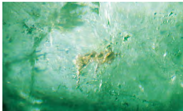
Figure 4. The filler (mixture of Epo Tek resins, R.I. = 1.550) in this 0.70 ct emerald appears brownish yellow. Photomicrograph by John I. Koivula; magnified 25 \times .
