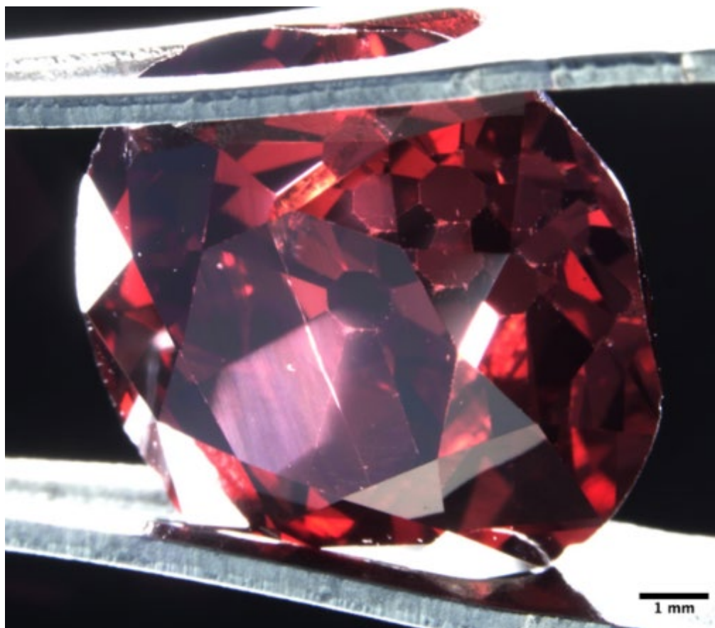
Figure S5. Major “feather” crack in the middle of the table appears to run parallel to one direction of graining.
