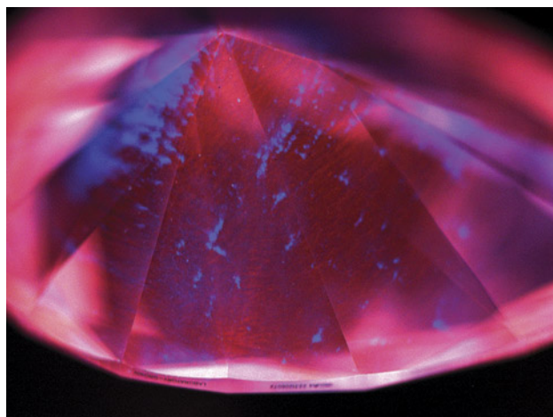
Figure 8. Representative deep-UV fluorescence image of a 2.90 ct CVD diamond from Plasmability, collected using the DiamondView. The image is dominated by red-orange fluorescence from NV^0 centers, a common feature for untreated CVD laboratory-grown diamonds, along with irregular blue fluorescing dislocation bundles. No growth layers were observed, indicating that it was produced through a single uninterrupted growth cycle. Image by Madelyn Dragone.
