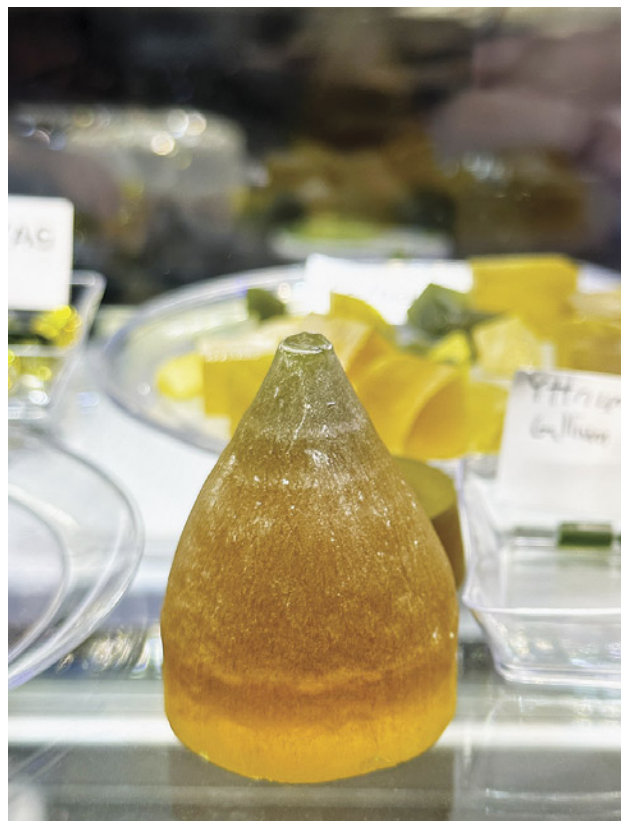
Figure 53. The top of a YAG boule doped with cerium and neodymium and produced by the Czochralski method, measuring approximately 36 mm in diameter and 45 mm tall. Parts of the boule that cannot be used for scientific purposes can be sold to the gem and jewelry trade for faceting. Photo by Lisa Kennedy; courtesy of Turtle’s Hoard.
