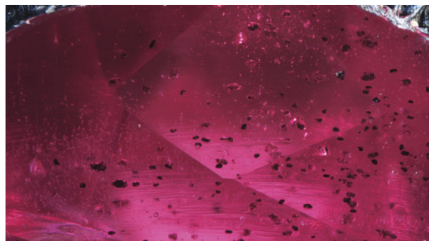
Figure 14. Strong curved growth lines and numerous gas bubbles and dark solid inclusions were present in the flame-fusion ruby. Photomicrograph by Ezgi Kiyak; field of view 2.9 mm.
