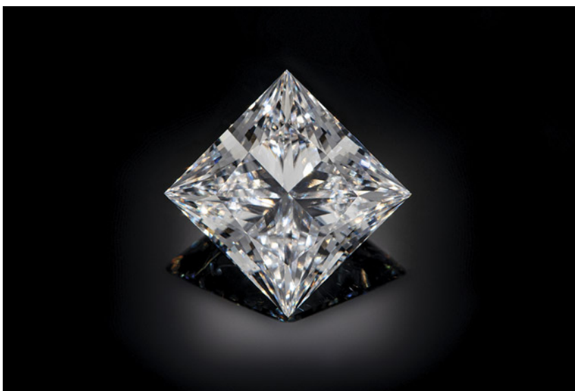
Figure 15. The new record size for CVD laboratory-grown diamond—16.41 ct, with G color and VVS 2 clarity—has been achieved by Shanghai Zhengshi Technology Co. Ltd. This is an as-grown diamond; no post-growth treatment was applied for color improvement, either before or after faceting.
