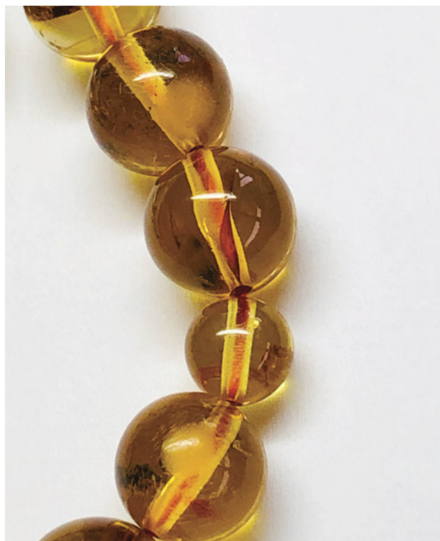
Figure 82. Epoxy resin is easily detected in the amber of this rosary. Photo by Nazar Ahmed Ambalathveetil.
