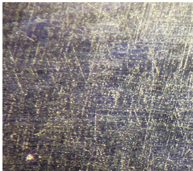
Figure 69. Needle-like inclusions arranged in four directions, viewed here from the top of the stone, created the asterism effect in the Vietnam topaz. Photograph by Le Ngoc Nang.
