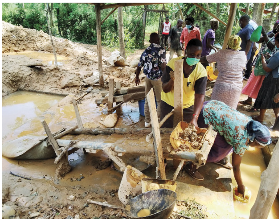
Figure 55. Miners wash the gold ores and use a sluice to collect gold within the slurry. Sluices are one of the most common tools used in artisanal and small-scale mining to concentrate gold. This simple configuration can capture ~20–70% of gold based on ore type, water flow, feed rate, and other specifications geometallurgists determine through research. Photo courtesy of Ruth Epwoka.
