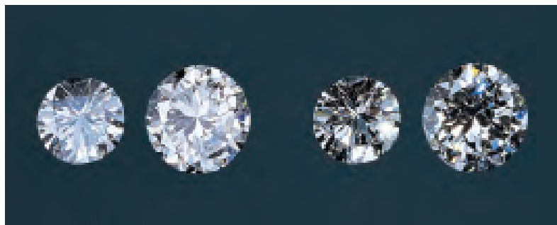
Figure 20. These two diamonds, with 50.7^\circ (RD27, left image in each pair) and 41.8^\circ (RD25, images at the right) pavilion angles, are neither bright (left pair, with diffuse lighting) nor fiery (right pair, with spot lighting). Composite of photos by Harold © Erica Van Pelt.
