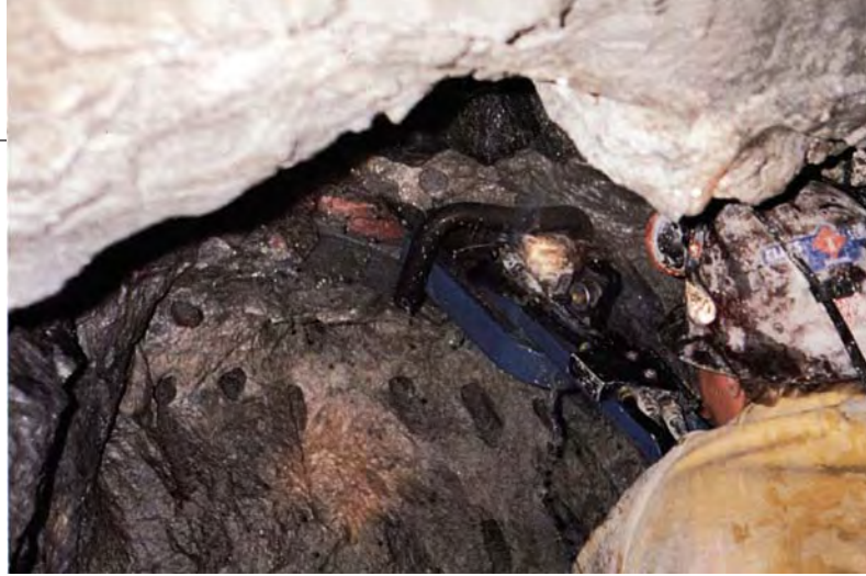
Figure 9. At Sweet Home, a miner used a hydraulic diamond-impregnated chainsaw to make the initial cut around a pocket. This pocket, recovered in 1994, was named the Corner Pocket, the source of many fine rhodochrosite specimens. Photo © Bryan Lees.
