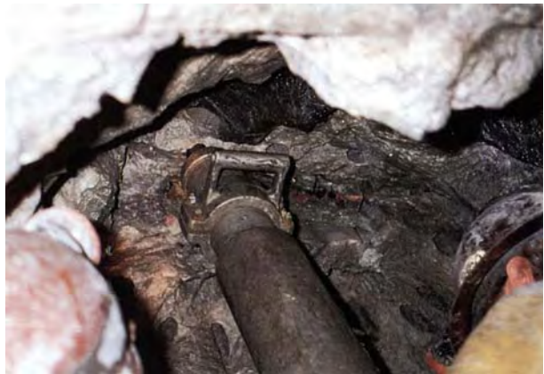
Figure 10. Two miners press upward with a splitter, a device similar to the “jaws of Life,” into holes drilled just outside the sawcut made around the Corner Pocket. Photo © Bryan Lees.
