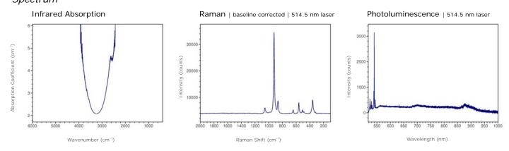
**Transmission infrared absorption spectra** were collected in the mid-IR range (400–6000 cm<sup>-1</sup>) using a Thermo-Nicolet 6700 FTIR spectrometer (KBr beamsplitter, MCT-B detector, 1 to 4 cm<sup>-1</sup> resolution, and 128 scans). A 6x beam condenser was used to focus light through the girdle region of the gemstone to obtain a maximum signal.
