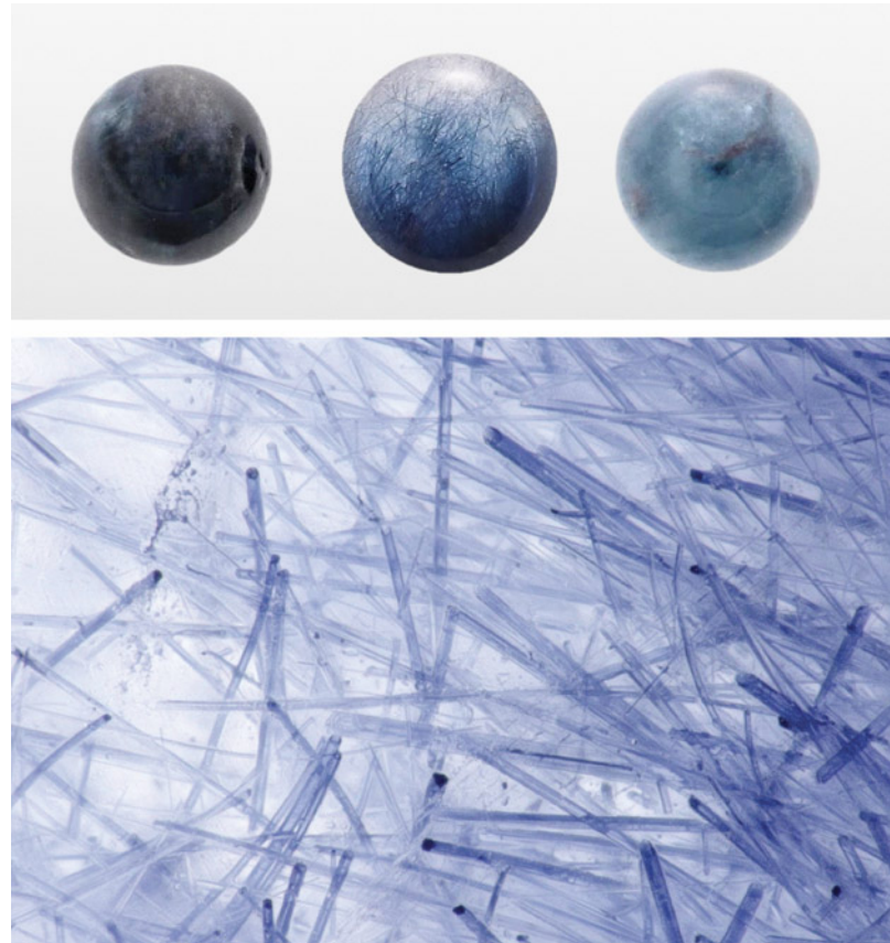
Figure 13. Top: Three quartz spheres weighing 4.85, 5.50, and 5.40 ct, respectively, colored by blue needle-like inclusions. Bottom: Abundant needle-like blue mineral inclusions in the 5.50 ct quartz sphere, with some displaying triangular cross sections; field of view 1.75 mm. Photos by Rong Liang.
