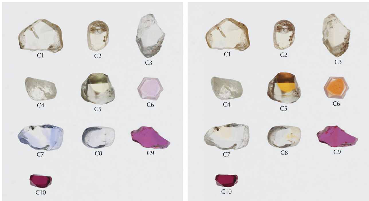
Figure 21. Color-calibrated photos of studied natural corundum crystals from various deposits ranging from 0.44 to 1.28 ct before (left) and after heating at 850°C (right). At this heating temperature, stronger yellow/orange coloration can be created. Photos by Sasithorn Engniwat.
