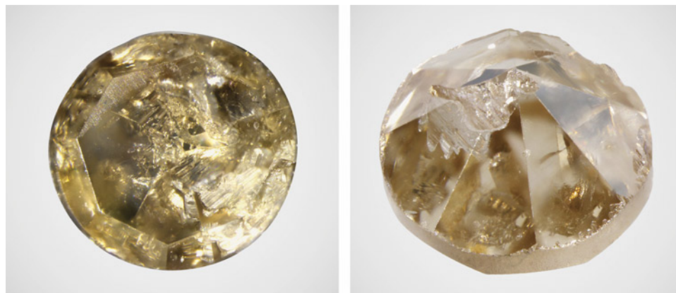
Figure 20. Table (left) and pavilion (right) views of the removed 0.0119 ct melee stone. Photos by Shunsuke Nagai.
