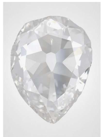
Figure 5. This 3.58 ct natural type IIa diamond with H color and SI 2 clarity displayed a unique fluorescence pattern when exposed to deep-UV light.
