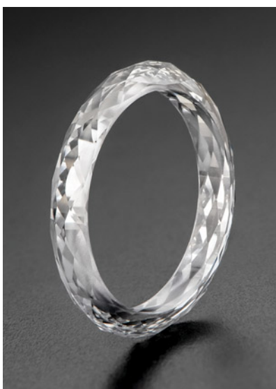
Figure 14. The 4.04 ct ring fashioned from a single-crystal CVD-grown diamond.
