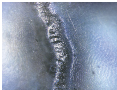
Figure 20. Rounded depressions forming the flame-like structure. Field of view 0.4 mm.
