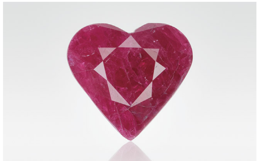
Figure 28. An 8.57 ct heart-shaped fracture-filled ruby treated with a zinc glass filling.
