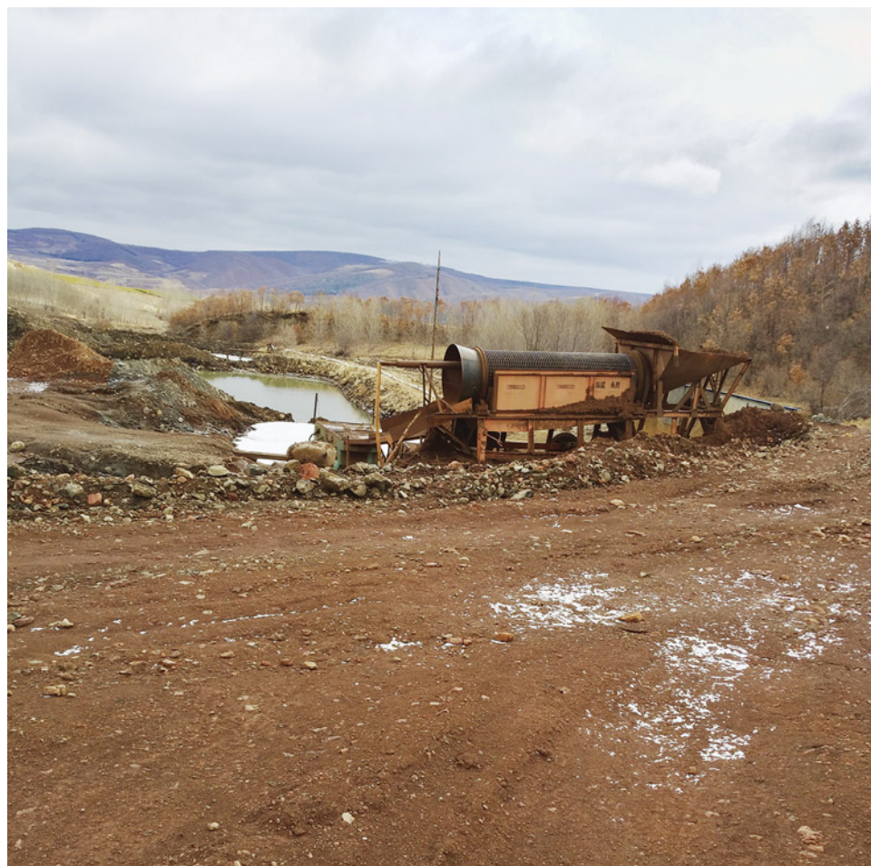
Figure 4. This photo of the Muling sapphire deposit, taken in April 2018, shows the trommel left unused. In this area, mining operations must cease for more than half the year because of freezing temperatures. The authors visited the mining site in June 2018, when weather conditions permitted mining activities. Photo by Aijun Yi.
