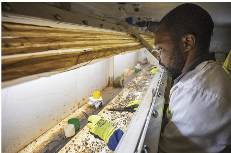
Figure 13. At GemRock, the concentrate from the wash plant is fed onto a conveyor belt where teams of sorters hand-pick the rubies. The workers are using glove-boxes to prevent physical access to the stones. At the end of the shift, the rubies are collected and inspected. Photo by Wim Vertrieft; courtesy of GemRock.
