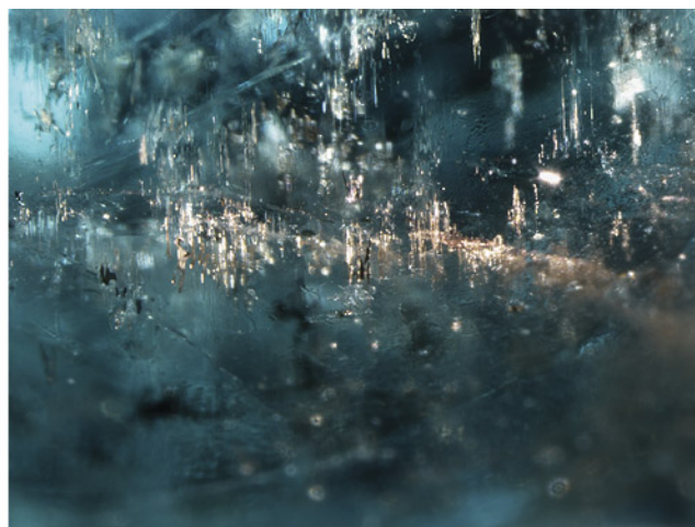
Figure 24. The copper inclusions aligned in the same direction appear brownish and black (left) and together display golden luster when the light enters from a certain direction (right). Field of view 2.3 mm.
