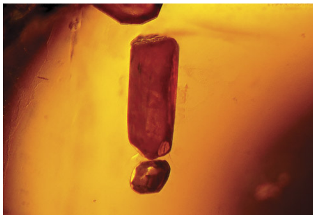
Figure 2. The “exclamation point” inclusions were identified as diopside crystals using Raman spectroscopy. Photomicrograph by Shu-Hong Lin; field of view 4.11 mm.
