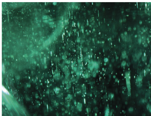
Figure 6. Internal features observed in the 2.99 ct Brazilian emerald. Left: Gota de aceite -like optical effect with columns resembling drops of oil. Note that this image was taken at an angle parallel to the c -axis. Right: Numerous raindrop-like needles and tubes. Fields of view 3.10 and 2.46 mm.
