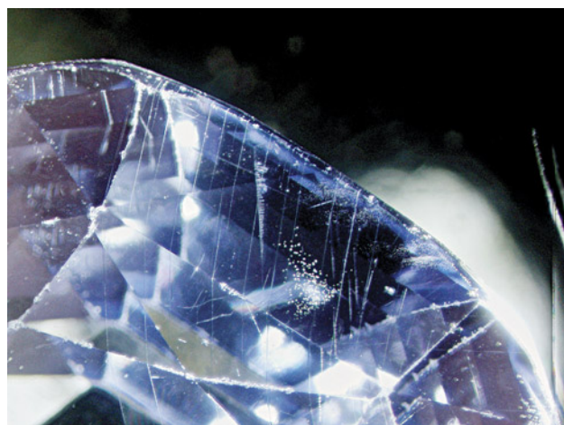
Figure 19. Clouds of bubbles, Rose channels, and twinning planes in the synthetic corundum. Photomicrograph by U. Hennebois; field of view 10 mm.
