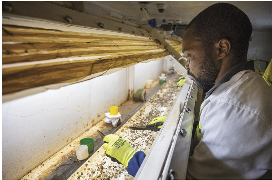
Figure 13. At GemRock, the concentrate from the wash plant is fed onto a conveyor belt where teams of sorters hand-pick the rubies. The workers are using glove-boxes to prevent physical access to the stones. At the end of the shift, the rubies are collected and inspected. Photo by Wim Vertriest; courtesy of GemRock.
