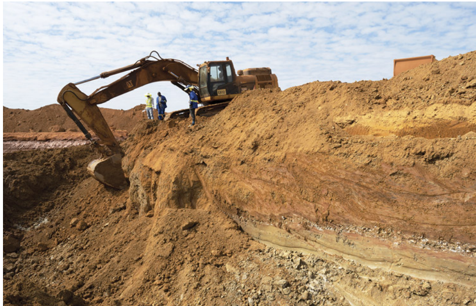
Figure 11. Mining of the gravels at Mugloto pit 3 in the MRM concession. The gravel layer is around 30 cm thick. The material on top has a distinct reddish tint that is typical for sediments in tropical environments. Under the layer of gravel, the weathered basement rock is more grayish in color. Photo by Wim Vertriest; courtesy of MRM.
