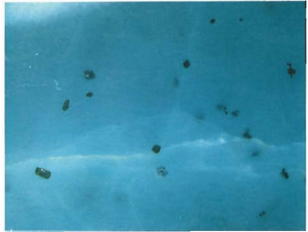
Figure 10. Rarely, minute euhedral monoclinic crystals of chalcocite are scattered in the blue pectolite. The presence of this copper sulphide strongly suggests that the color is related to traces of Cu. Photomicrograph by John I. Koivula; magnified 2 \times .
