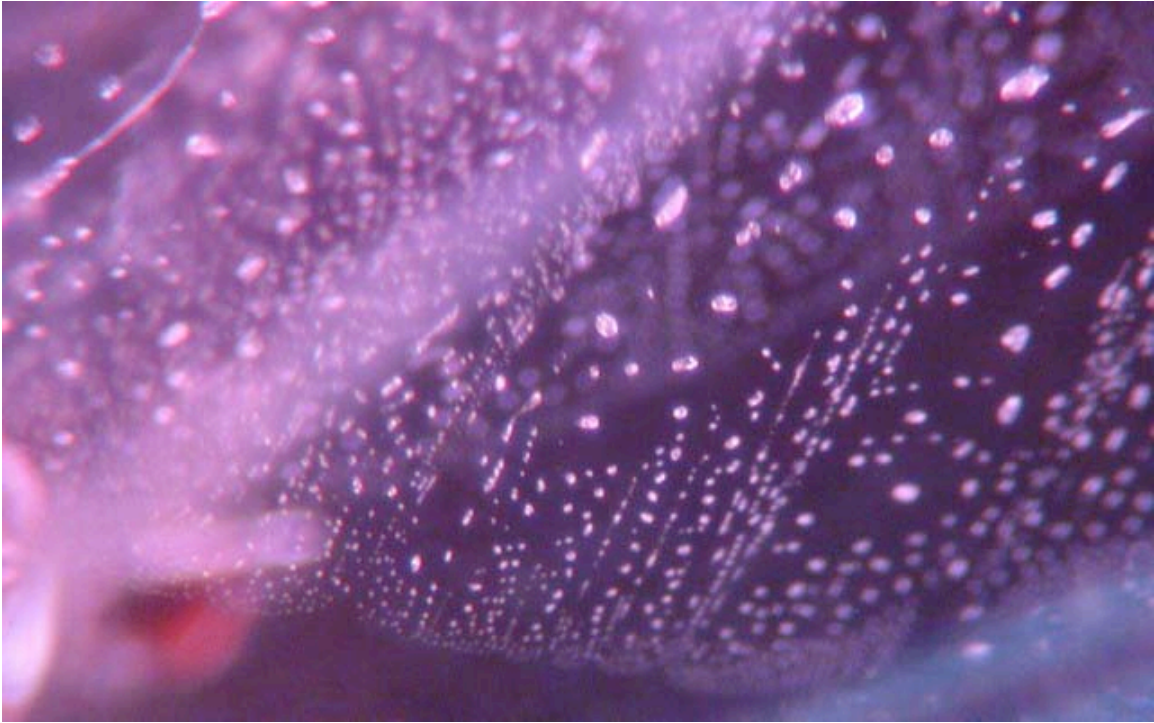
Figure DD-12. Partially healed fissure composed of negative crystals. Photomicrograph © V. Pardieu/GGL; magnified 20x.
