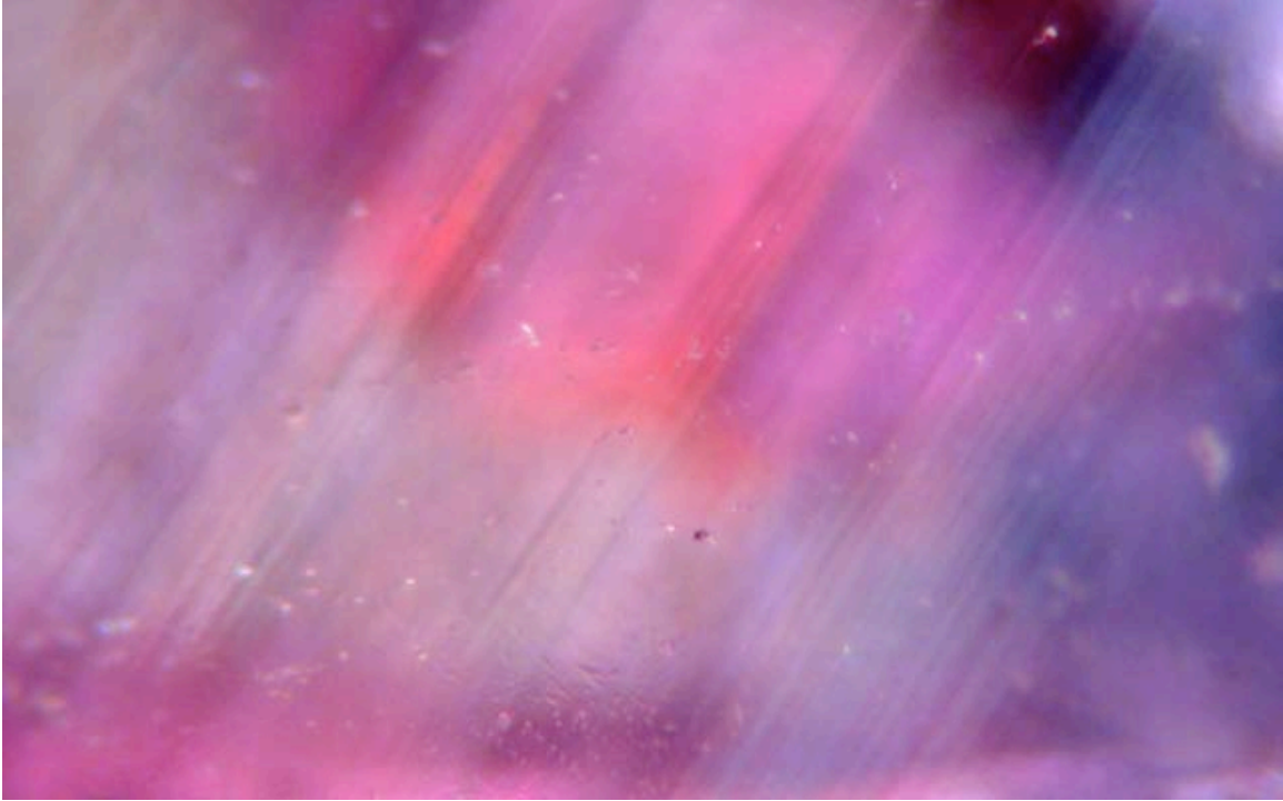
Figure DD-24. Bluish gray, slightly milky domains in the form of clouds, bands, or “growth sections” are common. In general, a milky appearance is caused by the presence of very tiny grayish pinpoints. Photomicrograph © V. Pardieu/GGL; magnified 20x, fiber-optic illumination.
