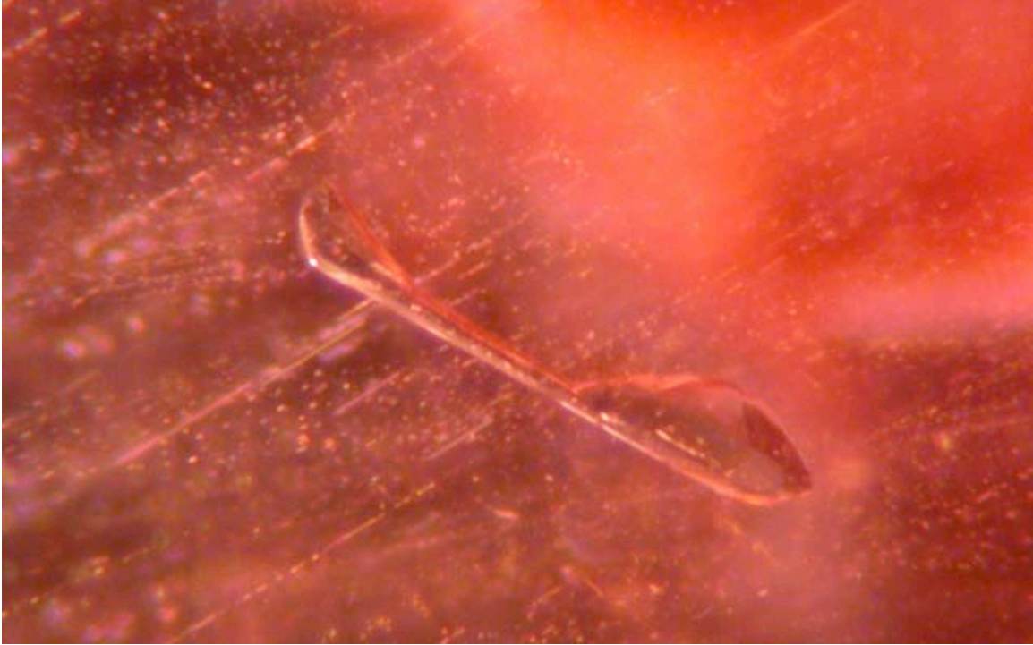
Figure DD-22. Elongate amphibole inclusion accompanied by needle-like formations that are oriented nearly parallel to one another. Photomicrograph © V. Pardieu/GGL; magnified 40x, fiber-optic illumination.
