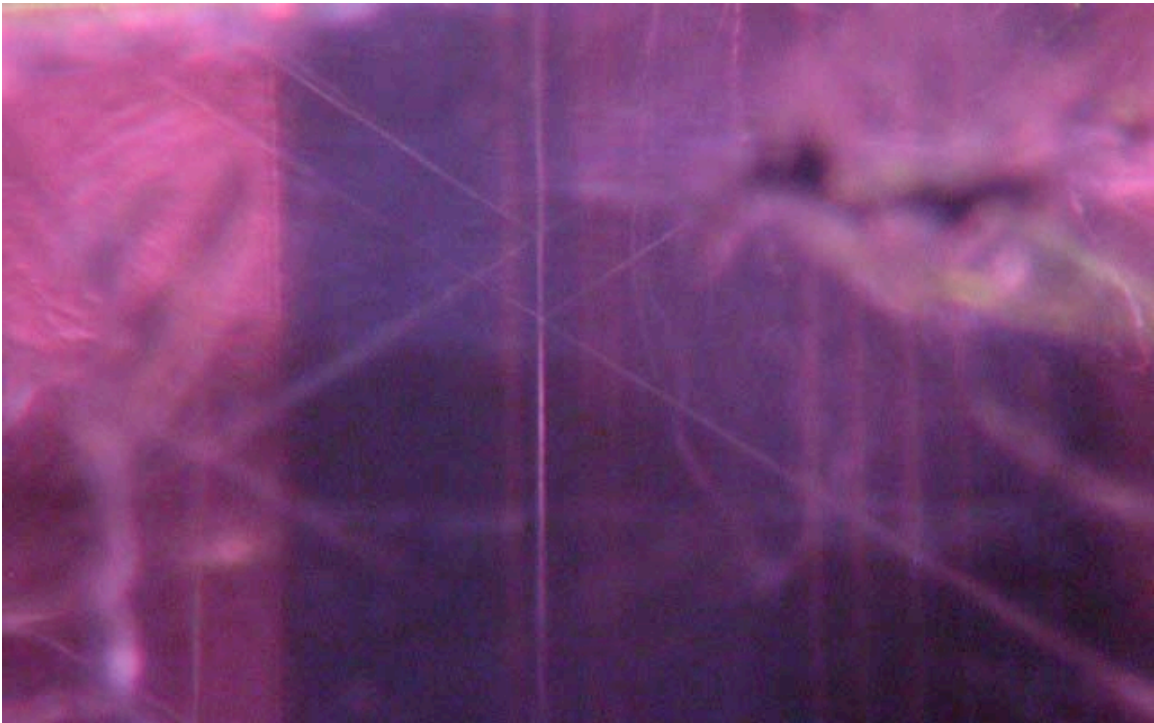
Figure DD-7. Intersection tubes and blue/pink color zoning. Photomicrograph © V. Pardieu/GGL; magnified 30x.
