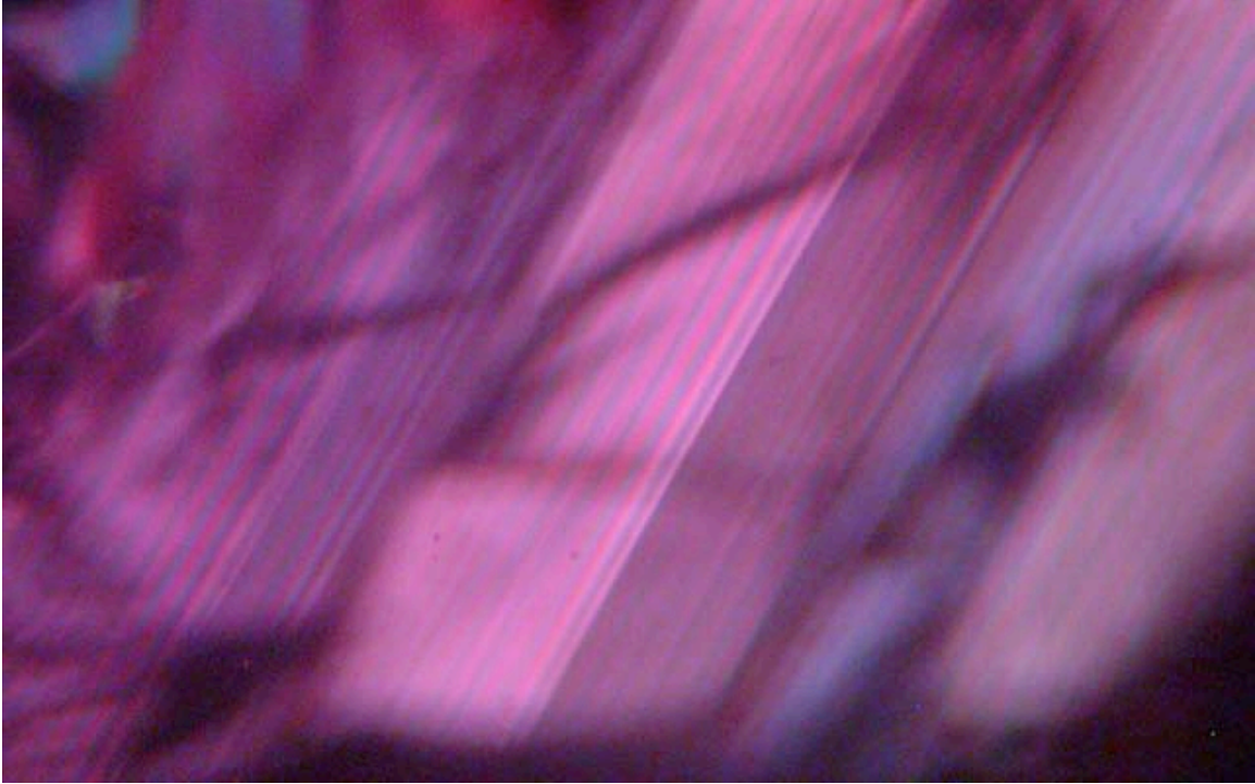
Figure DD-6. Twinning. Photomicrograph © V. Pardieu/GGL; magnified 40x, cross polars.
