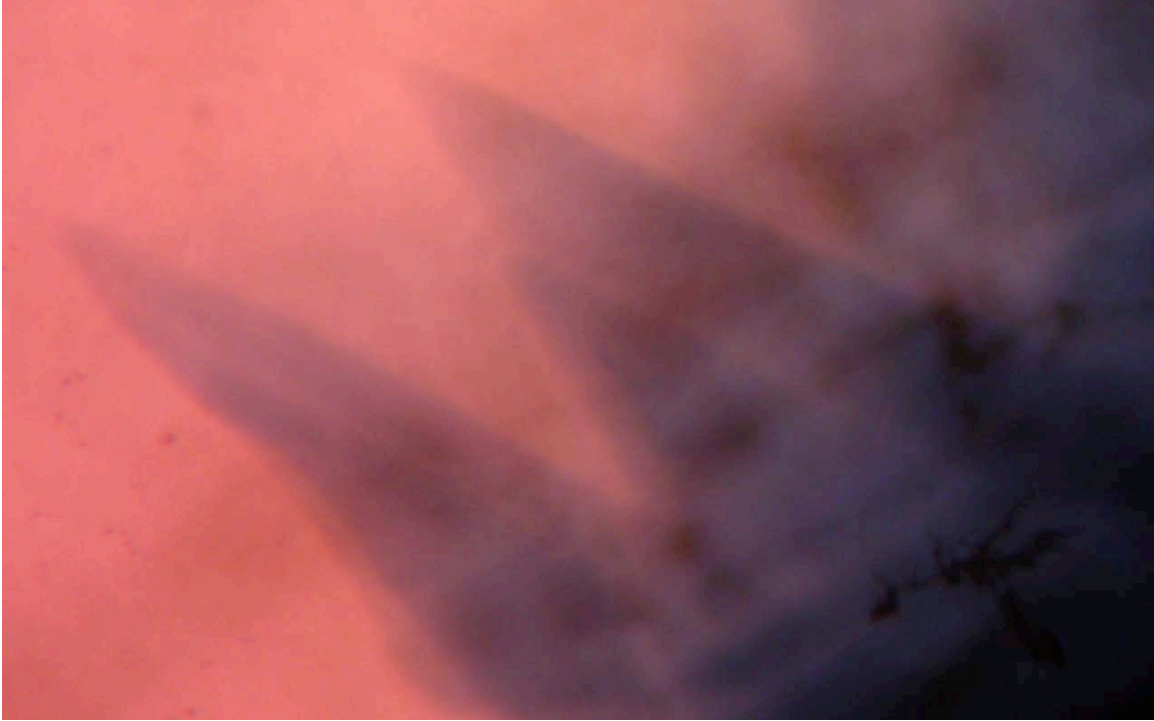
Figure DD-8. Color zoning. Photomicrograph © V. Pardieu/GGL; magnified 40x, brightfield illumination.
