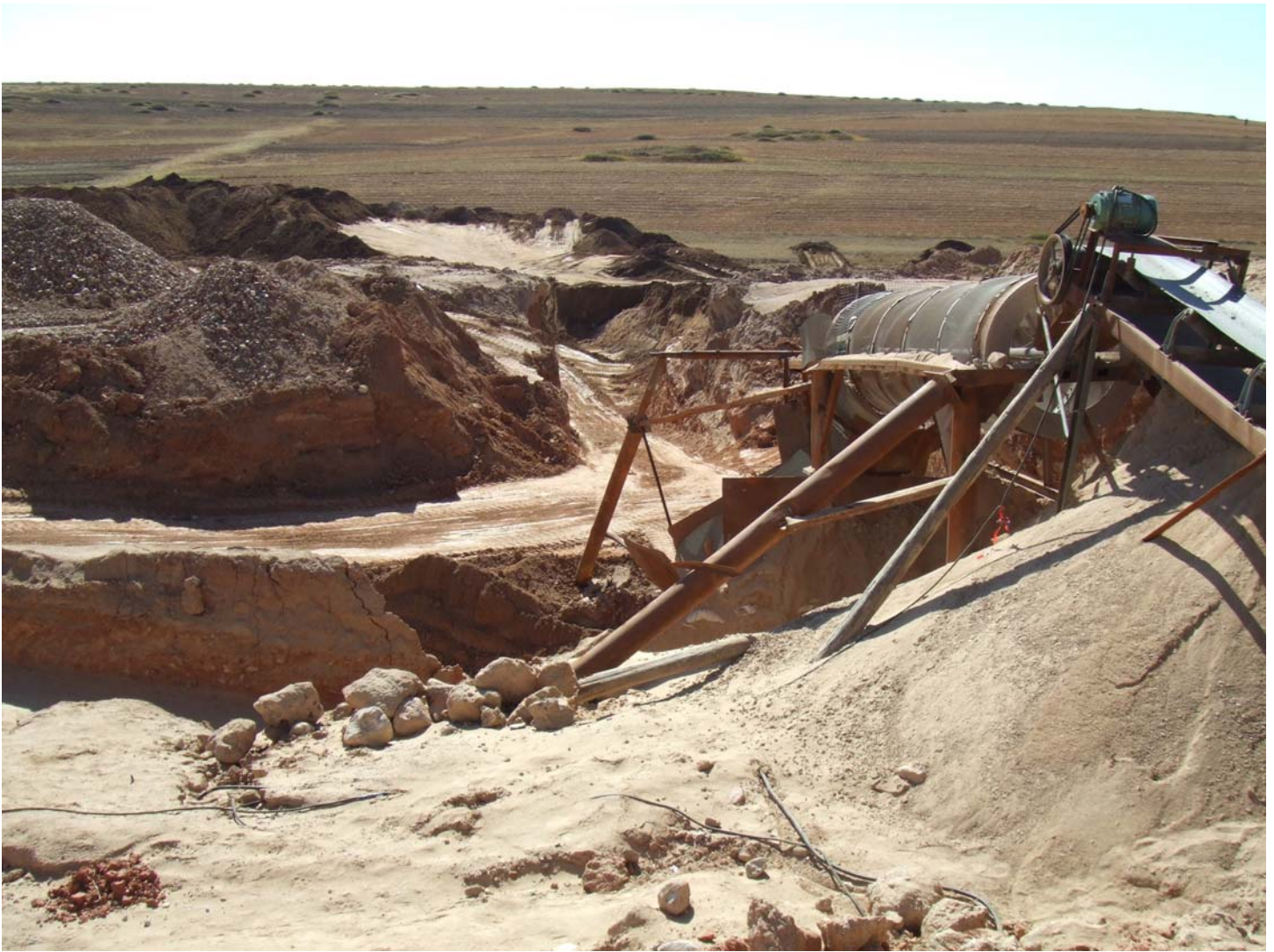
Figure DD-8. Rotating trommel at andesine mine in the Guyang area of Inner Mongolia. Photo by A. Abduriyim, © Gemmological Association of All Japan – Zenhokyo.
