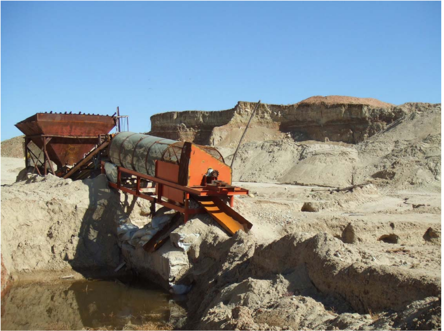
Figure DD-7. Rotating trommel at andesine mine in the Guyang area of Inner Mongolia. Photo by A. Abduriyim, © Gemmological Association of All Japan – Zenhokyo.
