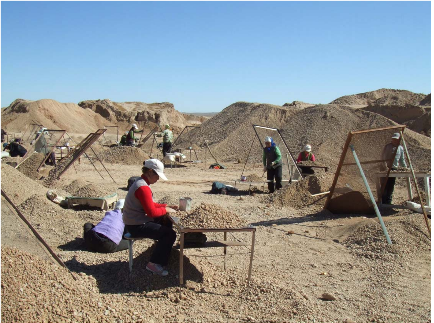
Figure DD-6. Andesine being recovered in Inner Mongolia using tilted screens. Photo by A. Abduriyim, © Gemmological Association of All Japan – Zenhokyo.
