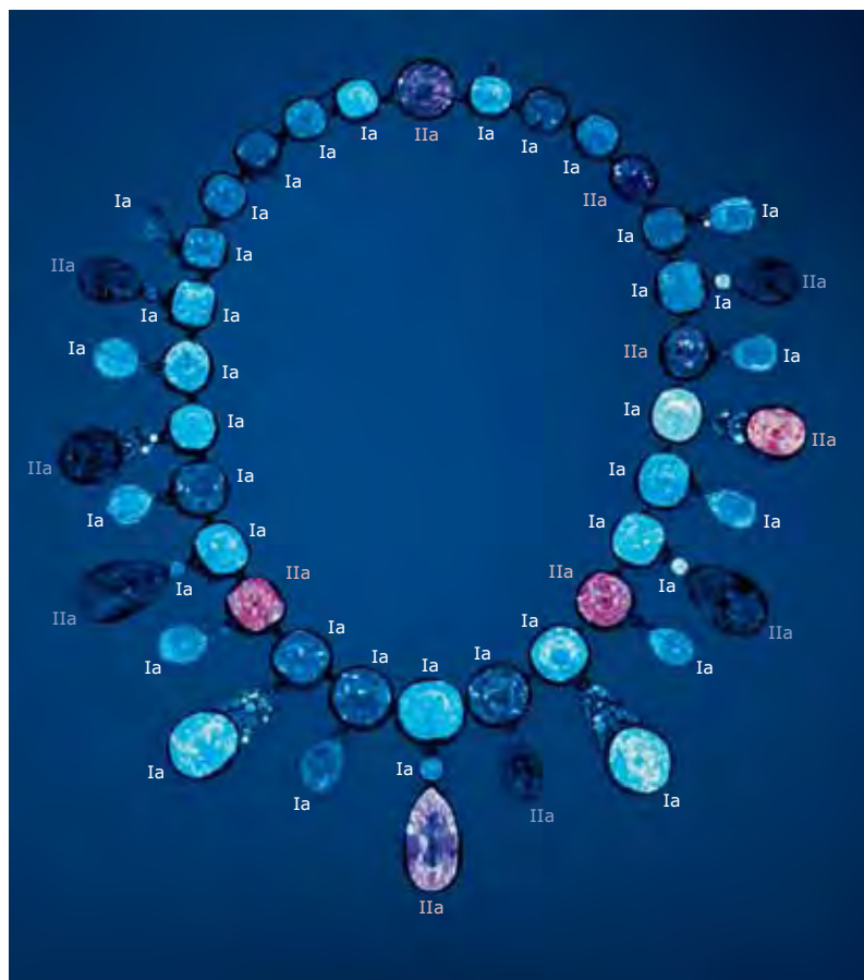
Figure 5. When the Napoleon Necklace is exposed to UV radiation (here, combined long- and short-wave UV), a variety of responses—pinkish orange, blue, or inert—can be observed. The diamond types, as determined by infrared spectroscopy, are labeled for the 52 larger stones; label colors correspond to the type of fluorescence: pink for pinkish orange, white for blue, and gray for inert. Photo by Chip Clark.
