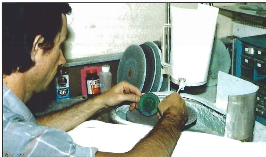
Figure 5. Polishing is the most time consuming—and potentially most hazardous—stage in the construction of fine intarsia. Should any one of the carefully chosen and matched pieces of banded malachite or patterned sugilite break, it could mean starting over almost completely on the project.
