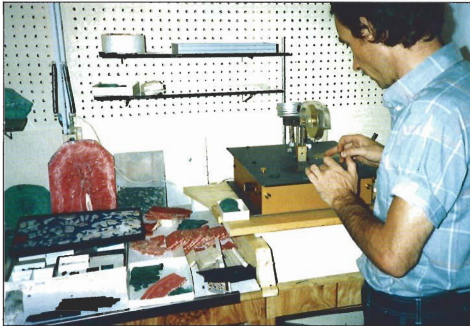
Figure 4. Once the slabs of malachite and sugilite were selected from several pounds of material, Medvedev proceeded to cut and trim the malachite to carefully fit the design of the box.
