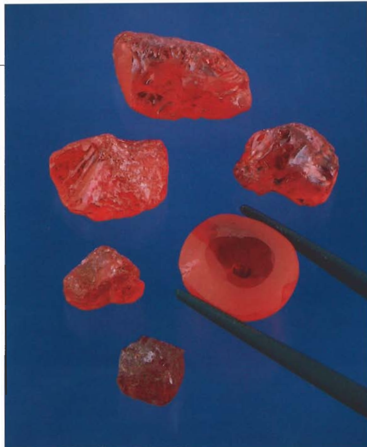
Figure 12. All six of these stones were purchased in Vietnam as natural ruby. On the basis of gemological testing and, in some cases, X-ray fluorescence analysis, the 11.44-ct preform and four of the pieces of rough (3.93–15.17 ct) were identified as Verneuil synthetic rubies; the smallest piece of rough (bottom, 3.79 ct) proved to be natural ruby. Photo by Shane McClure.
