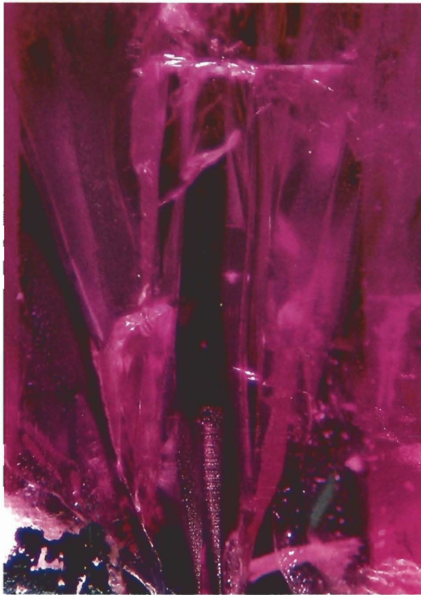
Figure 10. Various types of "fingerprint" inclusions and partly healed fractures originating from a central portion of a red beryl crystal. Dark-field and oblique illumination, magnified 20 \times . Photo by Robert Kane.
