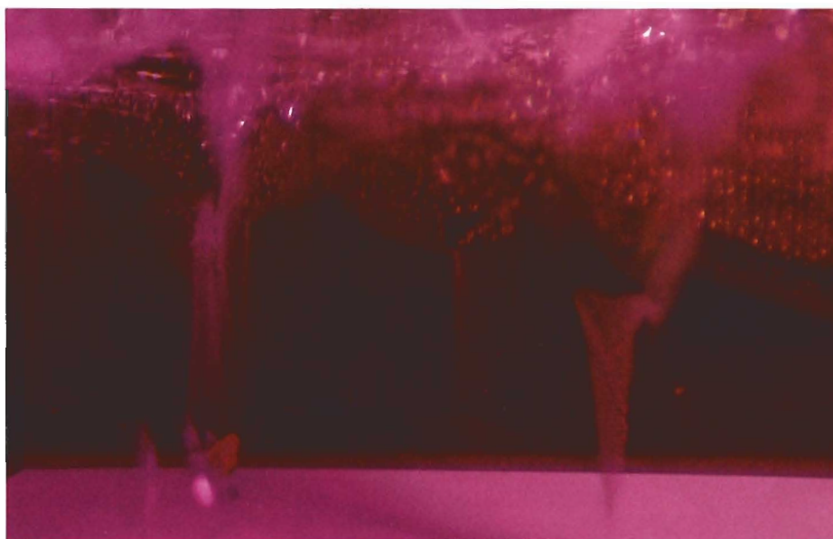
Figure 12. This faceted stone is host to dense concentrations of minute, white particles forming "comet tail" inclusions which are seen trailing behind "fingerprint" inclusions. Dark-field and oblique illumination, magnified 25 \times . Photo by Robert Kane.
