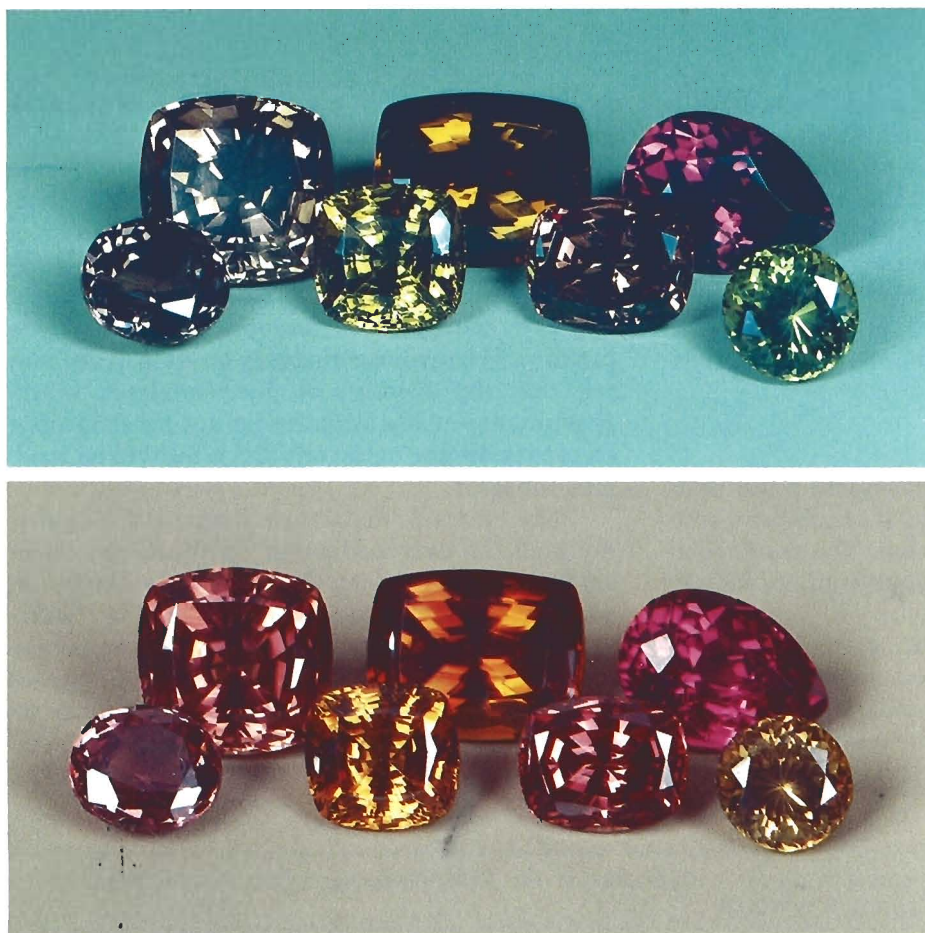
Figure 1. This selection of stones from the 32 garnets studied show the wide range of colors of this collection in both fluorescent (top) and incandescent (bottom) illumination. The GIA catalog numbers, from left to right, are 13433, 1009, 1055, 1023, 1043, 665, and 96A. The stones range in weight from 1.12 ct to 3.74 ct. Photos by Mike Havstad.
