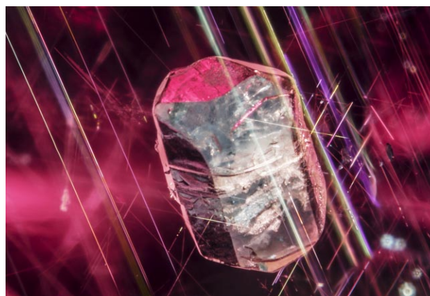
Figure 2. A blue apatite crystal associated with intersecting iridescent needles was showcased. Photomicrograph by Jessa Rizzo; field of view 2.90 mm.
