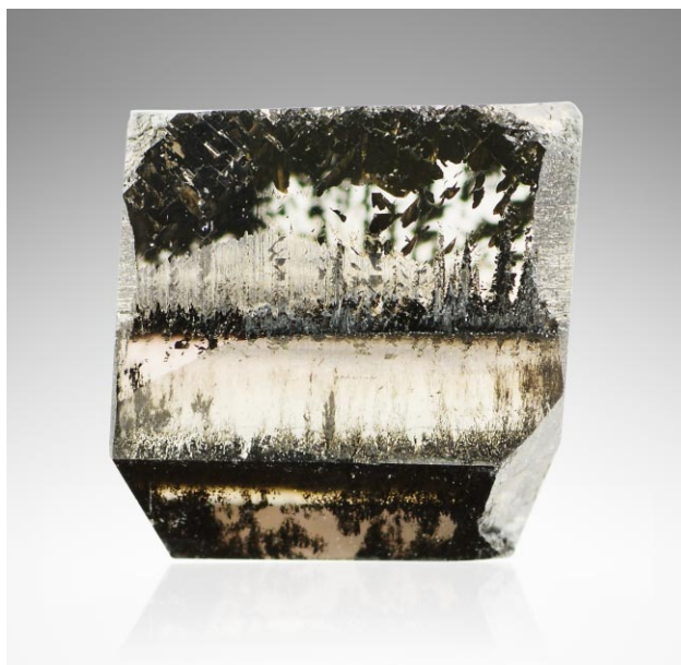
Figure 3. GIA-grown rough CVD diamond weighing 5.8 ct, photographed under daylight conditions. Photo by Towfiq Ahmed.
