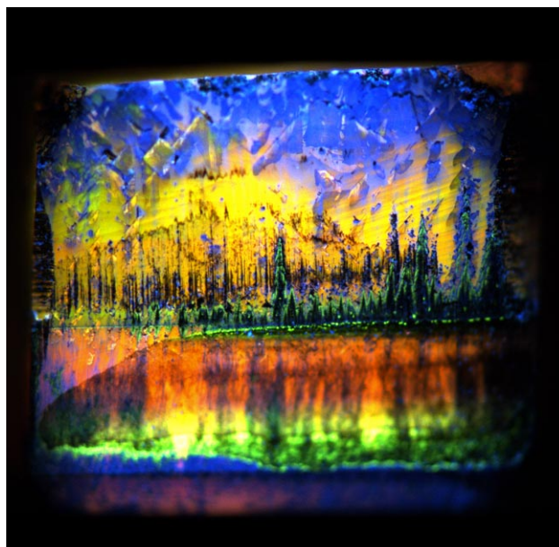
Figure 4. DiamondView fluorescence image of a 5.8 ct GIA-grown CVD block measuring 7 \times 7 \times 7 mm. Photomicrograph by Stephanie Persaud.
