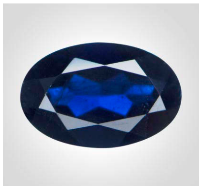
Figure 23. A 0.52 ct blue flux-grown synthetic sapphire.
