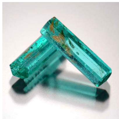
Figure 9. These two pieces of glass with copper inclusions, weighing 1.91 and 1.92 ct, appear to have been manufactured to imitate natural copper-bearing Paraíba tourmaline crystals.
