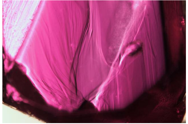
Figure 9. Roiled graining is consistent with a Mogok origin in this ruby. Photomicrograph by Charuwan Khowpong; field of view 2.83 mm.
