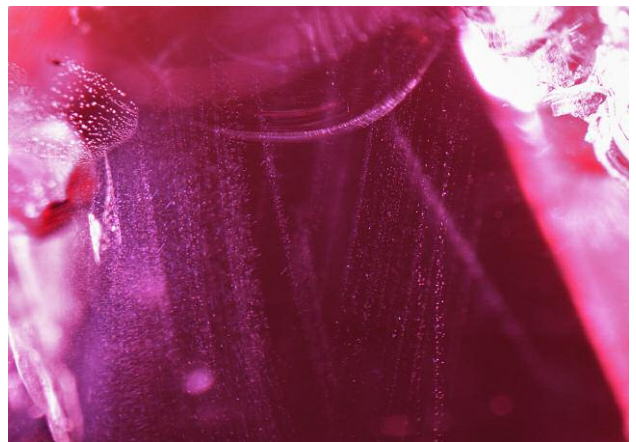
Figure 24. Stringer inclusions are also common in Afghan rubies. Photomicrograph by Charuwan Khowpong; field of view 3.1 mm.
