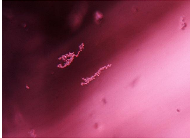
Figure 50. Clusters of small, rounded zircon crystals support a conclusive geographic origin determination for this Madagascar ruby. Photomicrograph by Patcharee Wongrawang; field of view 0.86 mm.
