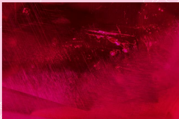
Figure CS 1-2. Nested straw-like silk and crystalline inclusions strongly suggest a Burmese origin. Photomicrograph by Aaron Palke; field of view 4.48 mm.
