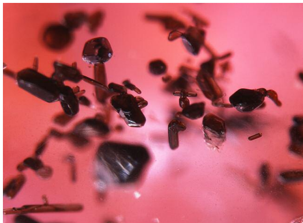
Figure 52. Blocky, euhedral rutile crystal inclusions are a common sight in Madagascar ruby. Photomicrograph by Patcharee Wongrawang; field of view 1.95 mm.
