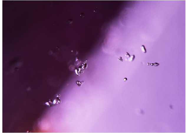
Figure 51. Madagascar rubies are often identified by clusters of small zircon crystals. Photomicrograph by Patcharee Wongrawang; field of view 1.56 mm.
