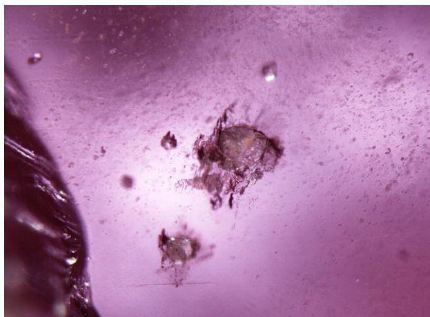
Figure 48. Muscovite inclusions, as seen in this Madagascar ruby, can also be found in Mozambique rubies. These inclusions alone should not be used to determine a ruby's geographic origin. Photomicrograph by GIA; field of view 0.97 mm.
