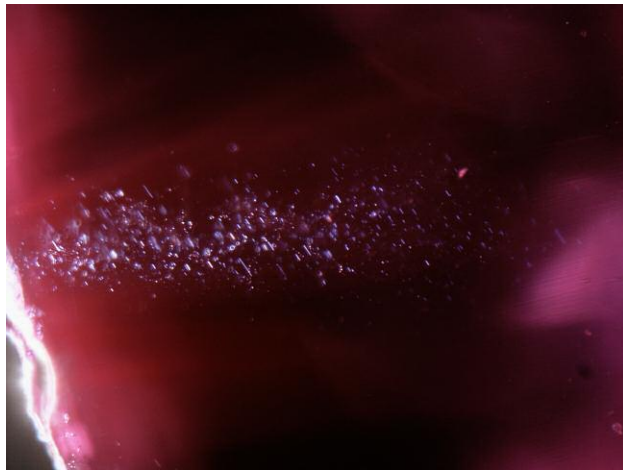
Figure 21. Short, thin rutile needles are also characteristic of Afghan rubies and may offer an indication of origin, along with other corroborating gemological data. Photomicrograph by Charuwan Khowpong; field of view 1.02 mm.
