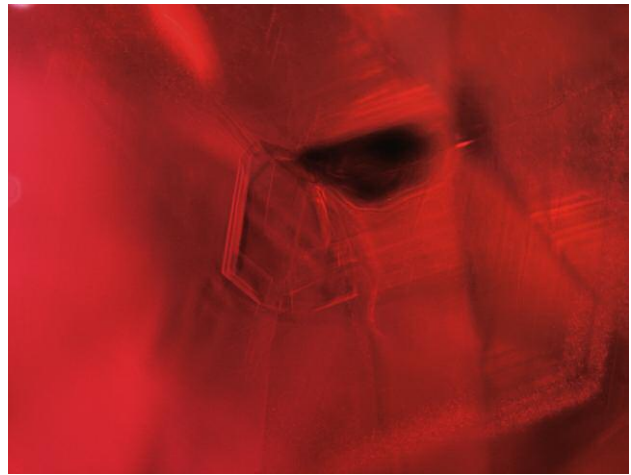
Figure 14. Stepped, angular graining can be seen in Mong Hsu rubies. Photomicrograph by GIA.
