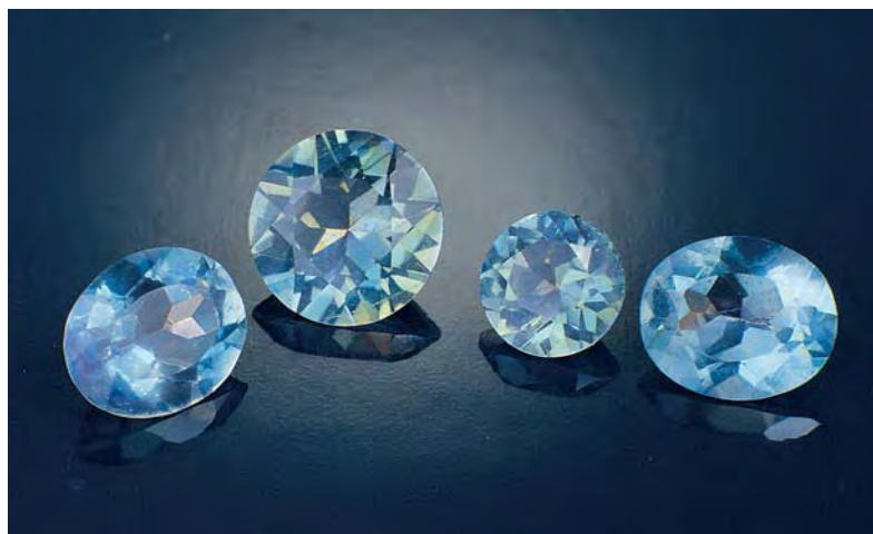
Figure 26. Aqua Aura treatment was still used extensively on quartz (the two inside stones) and topaz (the two outside stones) throughout the '90s. Photo by Robert Weldon.
