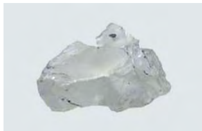
Figure 5. This 0.84 ct piece of type IIa diamond rough was HPHT annealed by General Electric for GIA researchers. The original dark brown material (left) was changed to approximately “G” color (right) after being subjected to the process. Photos by Elizabeth Schrader.
