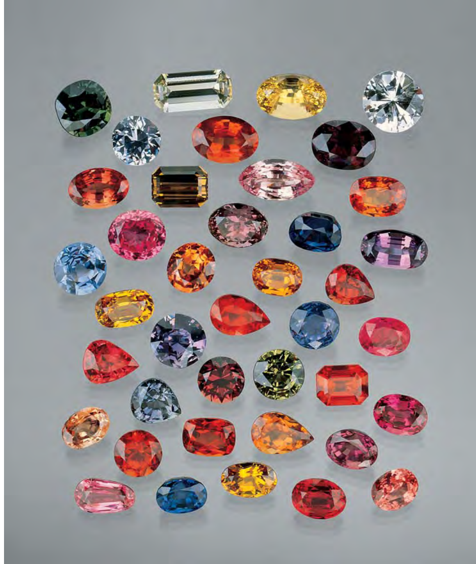
Figure 2. The vast majority of rubies and sapphires are now routinely heat-treated. The color or clarity (or both) can be improved in many different types of corundum by this process. Photo by Shane F. McClure.
