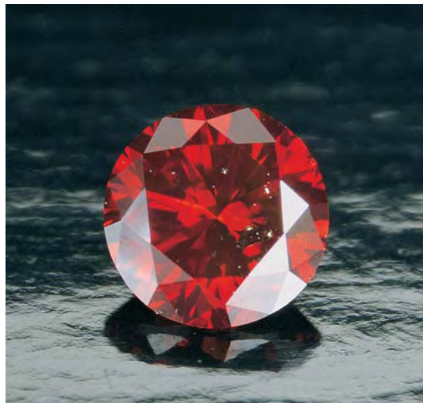
Figure 11. The red color in this 0.55 ct synthetic diamond was produced by irradiation and subsequent annealing. Photo by Robert Weldon.
