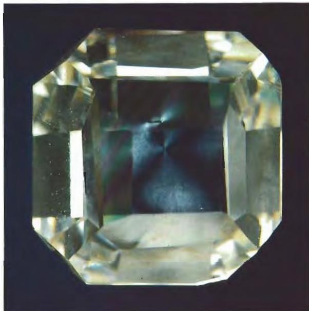
*Figure 6. A weak pattern of anomalous birefringence ("strain") can be seen in the smaller crystal when it is examined between crossed polarizing filters. The black, bluish gray, and light gray are low-order interference colors indicative of weak strain. The birefringence occurs around inclusions and in a pattern related to the arrangement of internal growth sectors. Photo by John I. Koivula.*
