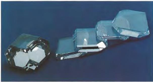
Figure 3. One of the new GE  $^{12}\text{C}$  synthetic diamond crystals is shown here cut into slices for use in various high-technology applications. Photo courtesy of General Electric.
