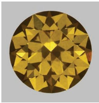
*Figure 1. This 0.88 carat synthetic nano-polycrystalline diamond was grown using a multi-anvil press by a new sintering process and faceted into a round brilliant stone. Photograph by Rob McMurtry.*
