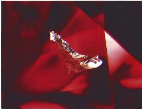
Figure 8. A deep cavity is evident in the table of the 0.95-ct diamond. When viewed from the pavilion, parallel angular growth steps can be seen. Darkfield illumination, magnified 35 $\times$ .
