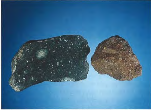
Figure 13. This photo clearly illustrates the effect weathering has had on Yogo sapphire-bearing rock. The greenish-gray sample of unweathered A-dike lamprophyre (from underground workings of the English mine) is composed of mica, pyroxene, analcime, and carbonates. The large circular feature is a carbonate-filled, pyroxene-rimmed vesicle; these vesicles were "bubbles" of an immiscible liquid within the Yogo magma. The reddish brown specimen is highly weathered material from the E dike within the Vortex mine; it consists of clays, carbonates, and some chlorite. After significant exposure to CO 2 -rich ground water, the greenish-gray specimen would eventually look like the reddish sample. Because it is much easier to process weathered dike material, Yogo sapphire miners still (as they did 70 years ago) expose large piles of hard, unweathered Yogo dike ore to rain, snow, and frost to accelerate the decomposition process. Photo by Maha DeMaggio.
