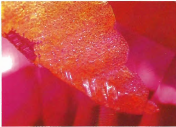
Figure 9. A distinctive orange to yellow color characterizes many of the flux globules and flux-filled voids in Ramaura synthetic rubies. The "crackled" appearance seen here is also quite typical of the Ramaura growth process. These flux inclusions can range from very rounded to very angular with straight, parallel steps. Dark-field and oblique illumination, magnified 35 \times .
