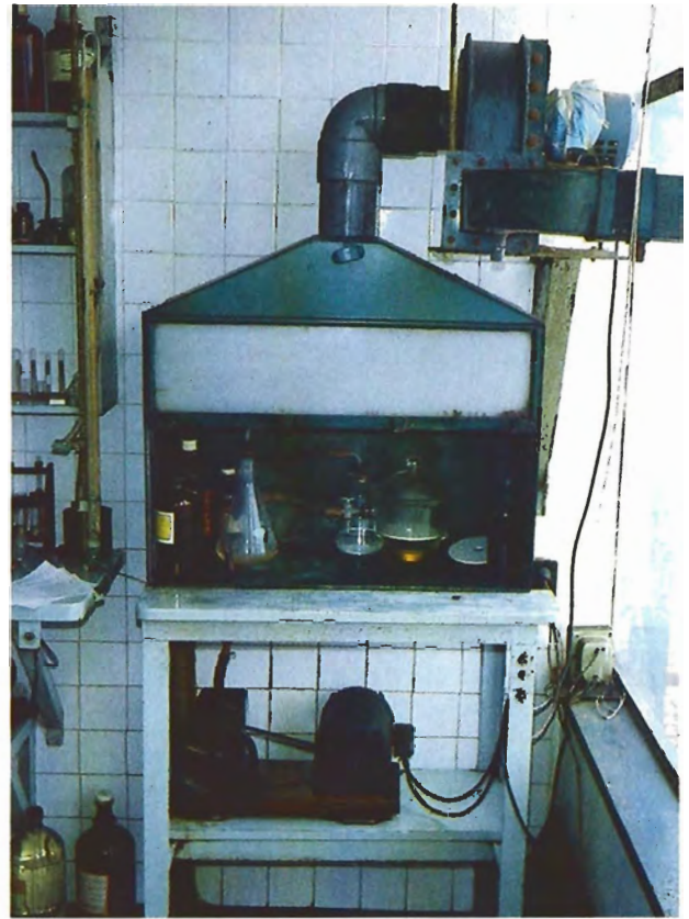
Figure 3. Fumes from the acid treatment are drawn away by this apparatus at Bargar Gemological Laboratories. The pump below draws a vacuum in the heated beakers.
