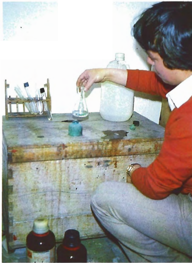
Figure 2. The alcohol used as fuel for the burner also serves as a solvent to clean the recently cut emeralds prior to treatment.
