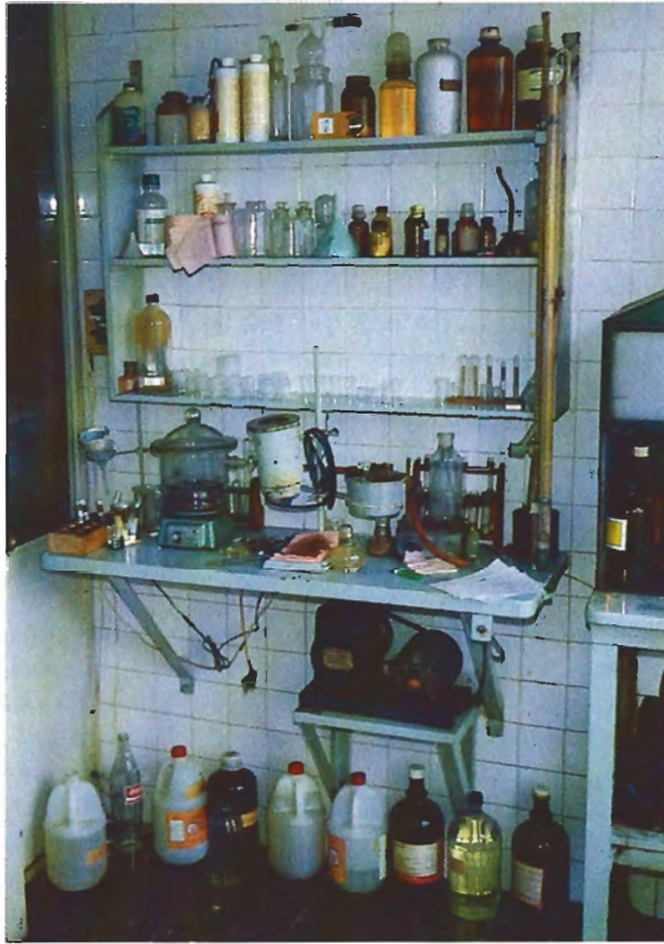
Figure 5. In Bogotá, Merck cedarwood oil is considered to be most effective for emerald treatment. In this apparatus at the Bargar Gemological Laboratories, the emeralds are soaked in the oil and then heated in a vacuum.
